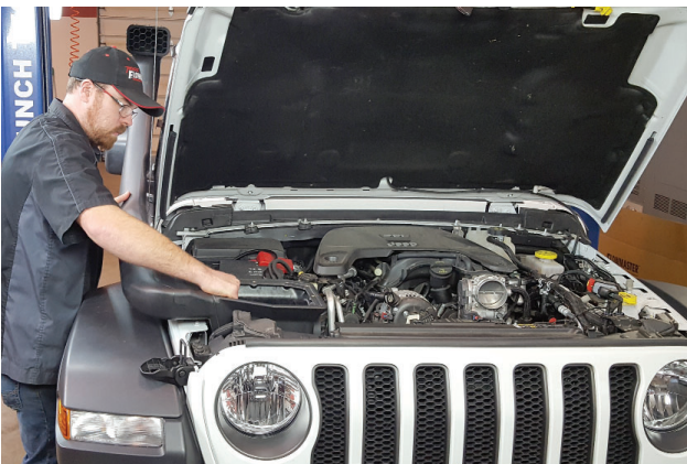
26. Place assembled airbox snorkel unit onto vehicle. Align air box into factory rubber grommets so it sets down in place.
