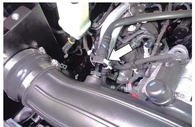
30. Connect the PCV line to the quick connect fitting and check for security.
