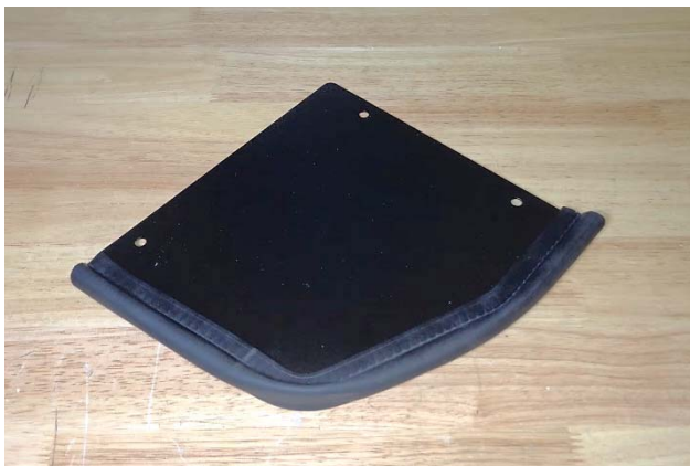
14. Attach gasket to the heat shield cover (5).
