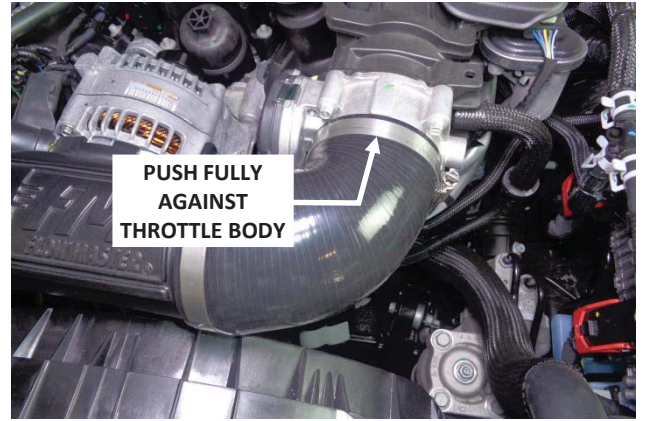
28. Push the elbow coupler up against the throttle body stops, then tighten the throttle body clamp.
