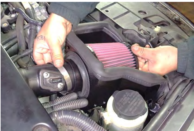
33. While holding the filter inside the heat shield, push the filter onto the intake tube, and press the heat shield's mount pin into the grommet in the vehicle frame. REPEAT ON THE DRIVER SIDE.
