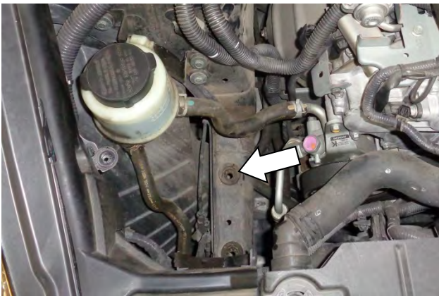
32. Before installing the heat shields, note that their barbed mount pins will be inserted in the rear mount grommets. (Moistening the grommets with soapy water will ease insertion.)
