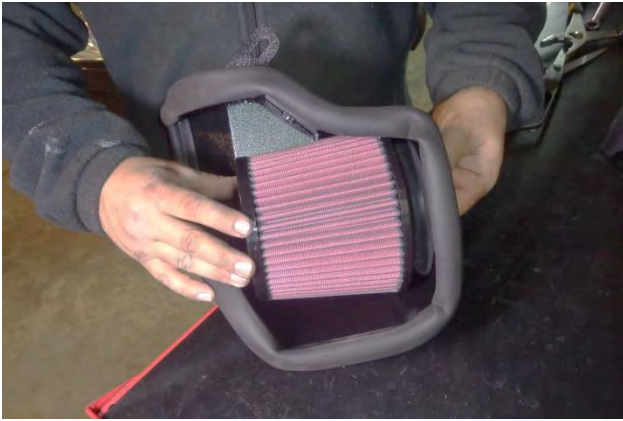
31. Carefully push the air filter flange through the heat shield opening. REPEAT ON THE DRIVER SIDE.
