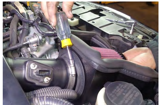
35. Adjust the alignment / rotation of the intake tube as required to obtain the best engagement with the coupler and the filter. Then secure the filter to the intake tube with the screw clamp. REPEAT ON THE DRIVER SIDE.
