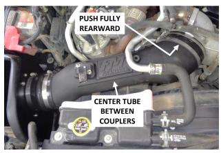
21. Install the assembled intake tube in the vehicle. Push the straight coupler up against the stops on the turbo inlet, then tighten the clamp. Then center the intake tube between the couplers, and tighten the last two screw clamps.
