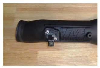
19. Slip the MAF sensor gasket (15) over the sensor, ensuring correct orientation. Then install the sensor in intake tube (11), using the M4 screws (16).
