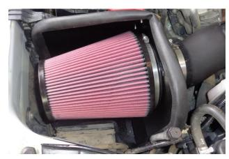
25. Install the clamp (2) on the air filter (1), then install the filter on the filter adapter and tighten the clamp.
