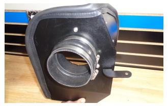
16. Slip the smaller screw clamps (9) onto the flex coupler (10). Install the coupler on the air filter adapter, pushing it flush against the heat shield. Tighten only the filter adapter clamp at this time. (Leave the other clamp loose.)
