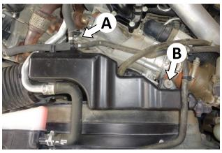
8. Loosen the screw clamp securing the intake duct to the turbocharger inlet (A). Then remove the intake duct mount bolt (B).
