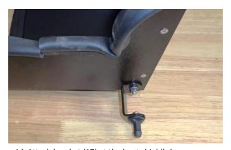
14. Attach bracket (17) at the heat shield's inner corner using a %-20  $\times$  5/8" screw (23) and flat washer (19) (against the heat shield), and a lock washer (20) and nut (21) (against the bracket). Then attach a barbed pin (14) to the bracket, using an M6 screw (8), lock washer (7) and flat washer (6).
