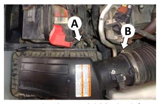
5. Remove the airbox mount bolt (A) and **retain for use at Step 18**. Then loosen the screw clamp securing the airbox to the intake duct (B).
