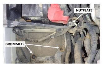
17. In the vehicle, identify the three points (two rubber grommets, and one nut-plate) to which the assembled heat shield will be mounted.
