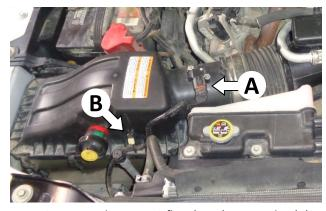
4. Disconnect the mass airflow (MAF) sensor plug (A) by pulling the locking tab away from the sensor until it stops, then squeezing the top and bottom of the plug and pulling it straight off the sensor. Then unclip the sensor lead from the airbox (B).
