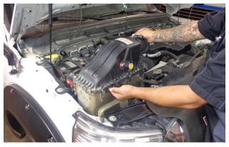
6. Separate the intake duct from the airbox, then firmly pull the airbox straight up to remove it from the vehicle.
