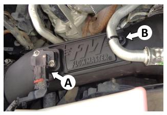
22. Reconnect the MAF sensor plug to the sensor (A), close the locking tab, and verify the connection is secure. Secure the metal tube to the intake tube (B) using cable tie (24).
