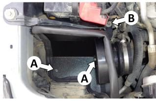
18. Install the heat shield in the vehicle by pushing the barbed pins into the rubber grommets (A). (Soapy water will ease insertion.) Then install **the stock bolt (B) removed at Step 5.** After tightening the bolt, tighten the bracket to the heat shield.
