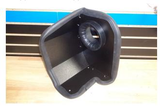
12. Firmly press the gasket (5) onto the edge of the heat shield, gradually working your way around. When you return to the starting point, use metal-cutting shears to trim the gasket to length.
