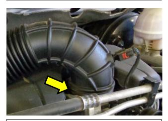
3. Loosen the hose clamp retaining the factory intake tube to the throttle body and remove the entire stock air-box/intake tube assembly from the vehicle by lifting straight up and out. Place the assembly on a flat stable surface for further steps.
