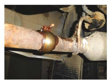
Locate the clamped connection just behind 1) each of the factory exhaust tips, spray the clamp bolt with a penetrating lubricant and allow to soak. Loosen the bolts and remove the factory tips from the vehicle.
