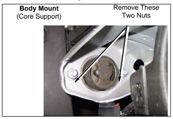
**d.** Passenger Side: Remove bolt and lower bushing from each cab mount on passenger side. 2
