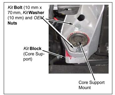
**g.** Install *kit* **blocks** (2" x 3") onto factory body bushings on each body mount.
