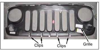
**b.** Install six screw clips along top of grille.
