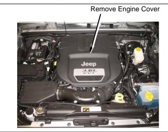
e. Remove two air hose bolts and loosen screw clamps from throtle body and air box; then remove air hose from engine bay.
