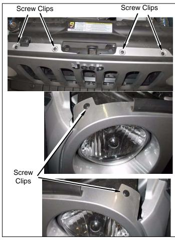
**c.** Remove grille from vehicle by popping four clips along bottom of grille.
