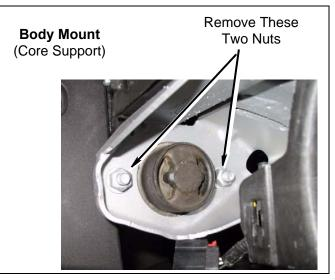
b. Driver Side: Loosen, but DO NOT REMOVE, body mounting bolts. 2 & 4 Door have four body mount bolts.
