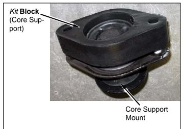
f. Install four *kit* washers (10 mm), two *kit* bolts (10 mm x 70 mm), two OEM nuts (10 mm) and core support mount on vehicle.
