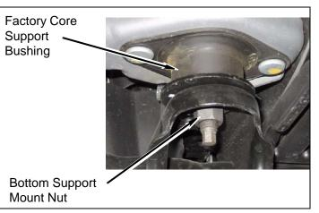
c. Remove core support bushing from vehicle.
