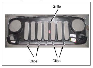
**b.** Install six screw clips along top of grille.
