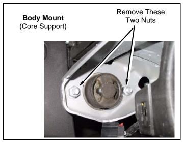
b. Driver Side: Loosen, but DO NOT REMOVE, body mounting bolts. 2 Door - 4 body mount bolts and 4 Door - 5 body mount bolts.
