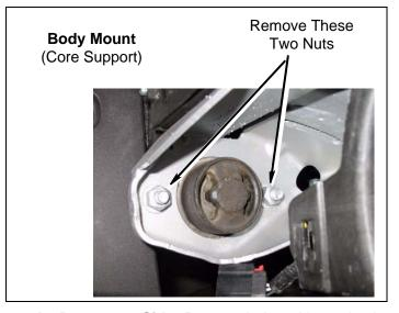
d. Passenger Side: Remove bolt and lower bushing from each cab mount on passenger side. 2
