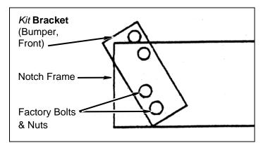
b. Cut two front factory bumper brackets for clearance with frame and factory bumper hardware as shown.
