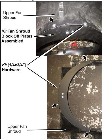
j. Using second pair of kit fan shroud block of plates. (Leave brackets slightly loose until mounted onto fan shroud, this will allow you to adjust the plates as needed to fit shroud properly.) With both kit fan shroud block off plates assembled, face the tabs outwards so that the kit fan shroud block off plate assembly mounts evenly with the inside edge of the lower fan shroud assembly. (Tighten assembly now.)
