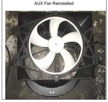
m. Carefully reinstall engine fan & fan shroud back into lower locking tabs and engine fan clutch back onto engine water pump pulley with correct tooling.
