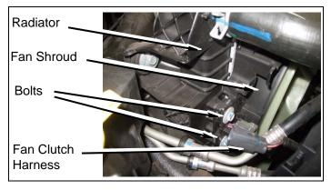
Locate factory lower fan shroud insert shield and remove lower fan shroud insert shield.
