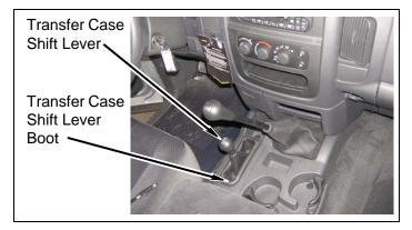
d. Remove cup holder inserts, three screws, and center console from floor.
