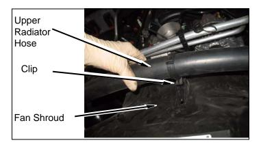
b. Remove fan shroud wire harness to AUX fan. Remove two bolts from fan shroud and prepare to remove fan shroud with engine fan. (Note: Only if equiped with AUX fan.).
