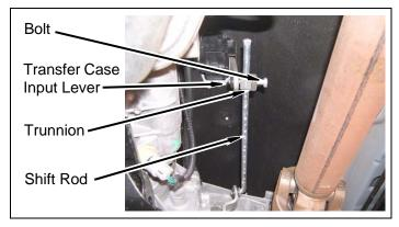
c. Verify the 4WD shift lever operation. Ensure there is complete engagement in all ranges. It may be necessary to adjust the position of the trunnion on the shift rod to obtain proper engagement in all ranges.
