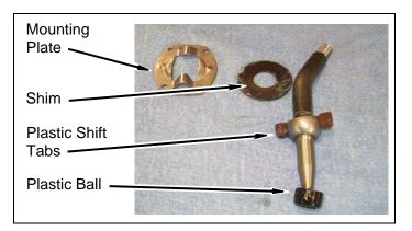
Scribe a line along side of transmission shift lever (below lowest bend). Measure diameter of shift lever (below lowest bend). Cut lever into two pieces and deburr as necessary.
