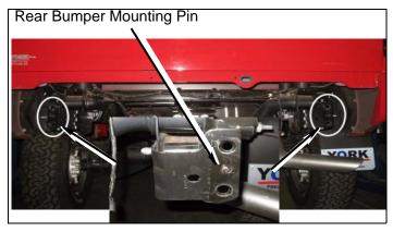
c. Apply small amount of kit Loctite® onto threads of factory bolts. Install two kit brackets (rear bumper) onto frame and bumper with two factory bolts and nuts with captive washers and two kit bolts (1/2" x 1-1/4") and install rear bumper onto kit bracket (rear bumper, middle) with two kit bolts (7/16" x 1-1/2"), four kit washers (7/16" USS), and two kit nuts (7/16" Nylock). DO NOT TIGHTEN.
