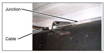
c. Remove front parking brake cable from driver side parking brake cable mount.
