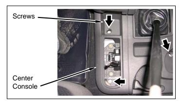
e. Unscrew transmission shift lever from shift tower.
