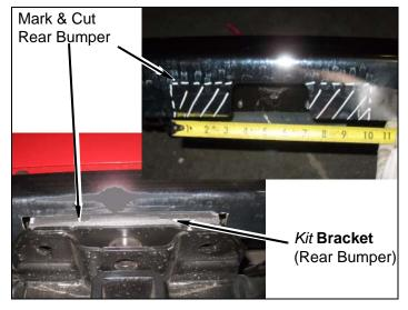
e. Apply small amount of kit Loctite® onto threads of two *kit* **bolts** (7/16" x 1-1/2") and install rear bumper onto *kit* **bracket** (rear bumper, middle) with two *kit* **bolts** (7/16" x 1-1/2"), four *kit* **washers** (7/16" USS), and two *kit* **nuts** (7/16" Nylock). DO NOT TIGHTEN.
