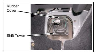
h. Install shift lever boot seal onto floor with six bolts.
