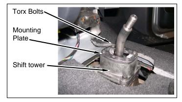
g. Install rubber cover onto shift tower.
