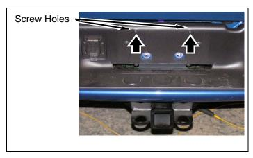
c. Remove two bolts from center of bumper.
