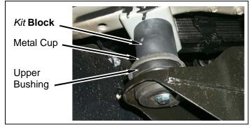
d. Lower passenger side cab onto kit blocks.
