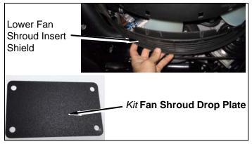
c. Using a pair of visegrips or clamps; create a 3" gap at the center of the fan shroud by separating & squaring the main engine fan shroud with the lower fan shroud insert shield; then clamp the assembly together using two kit side shroud drop plates at each side.
