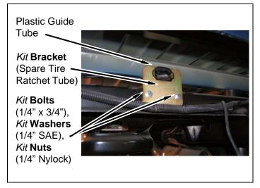
i. Install ratchet tube onto spare tire winch with retaining clip.
