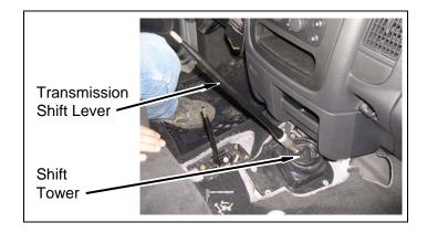
Remove six bolts and shift lever boot seal from floor.
