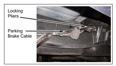
b. Use expanding pliers and disconnect parking brake cable from junction.
