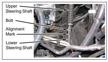
c. Remove bolt and slide upper steering shaft up to separate from lower steering shaft.
