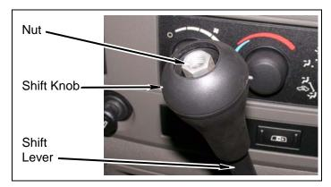
c. Remove transfer case shift lever boot from center console.
