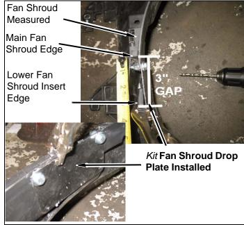
d. Once you have shaped and placed each kit fan shroud drop plates into place; reclamp and secure each kit shroud plate at a 3" gap and mark each 1/4" holes for drilling.
