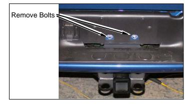
d. Remove four bolts from bumper and frame.
