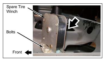
Install kit bracket (spare tire winch) onto crossmember with factory driver side bolt. DO NOT TIGHTEN.
