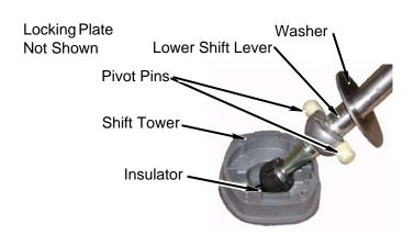
2. **4WD Models:** Remove the shift transfer case shift linkage.
