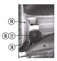
2. Lift cab and install cab passenger side spacer blocks.
