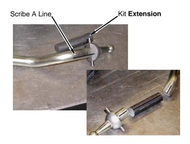
b. Position kit **extension** transmission shift lever 5/8" x 3" between two pieces of transmission shift lever. Ensure kit **extension** and shift lever scribe lines align and weld extension in place. Let shift lever cool.
