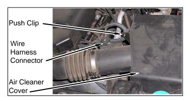
b. Remove two clips, hose clamp, and air cleaner cover from air cleaner base.
