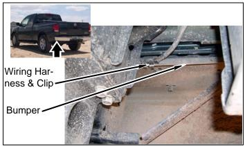
b. Remove three wiring harness push clips from rear bumper bracket.
