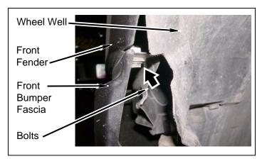
Install front bumper fascia onto driver and passenger wheel wells with six screws.
