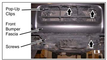
c. Remove six screws from driver and passenger front bumper fascia and wheel wells.
