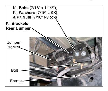
h. Install kit **bracket**, **hitch support** on hitch and rear bumper with four kit **bolts** (7/16" x 1-1/2"), eight kit **washers** (7/16" SAE), and four kit **nuts** (7/16" nylock).
