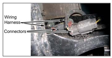
d. Remove two license plate light connectors from rear bumper.
