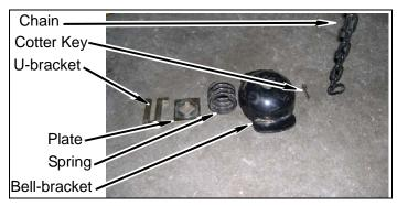
b. Position chain through, and position winch mechanism on top of frame cross member with kit **bolt** (M10-1.25 X 100mm) and kit **tube spacer**. Do not tighten. Mark where chain contacts frame cross member and remove winch mechanisism.
