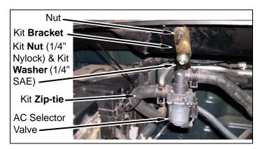
d. Install kit **zip-tie** on hose of AC selector valve and electrical control box as shown.
