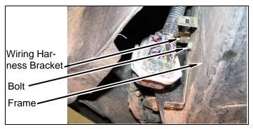
Remove two wiring harness push clips and wiring harness from frame / body mount perch.
