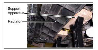
b. Mark and cut lower radiator support and ribs as shown.
