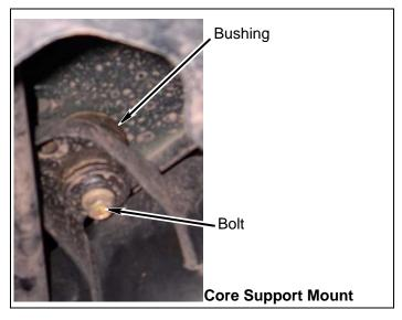
b. Remove three bolts from cab bushings on passenger side.
