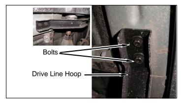
b. Reposition catalytic converter ground strap on body so end link connector is pointing forward.
