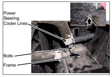
b. Remove clip and wiring harness from frame.
