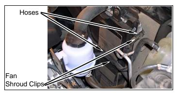
c. Remove two bolts and fan shroud from radiator. Lift and remove fan shroud from vehicle.
