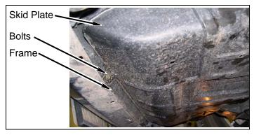
If equipped, remove four bolts and two tow hooks from frame.
