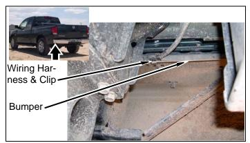
b. Install and connect two wiring harness connectors on rear bumper and wiring harness.
