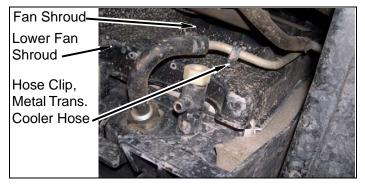
b. Remove transmission cooler hose and lower fan shroud from fan shroud and vehicle.
