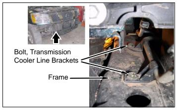
d. Remove clip and wiring harness from frame.
