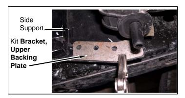
f. Install lower radiator support assembly and kit bracket, upper backing Plate on side supports with six kit bolts (1/4" x 1"), twelve kit washers (1/4" SAE), and six kit nuts (1/4" nylock).
