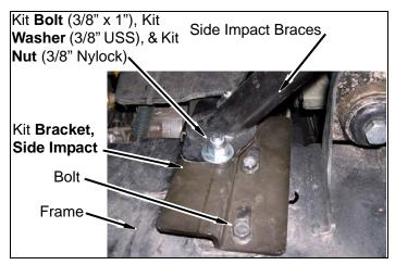
c. Mark and cut two side bumper braces as shown.
