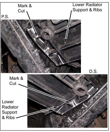
c. Position and mark twelve holes from kit **brackets**, **upper radiator support** on lower radiator support. Drill 1/4" holes where marked.
