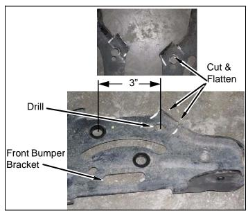
d. Install two modified front bumper brackets on frame with four bolts.
