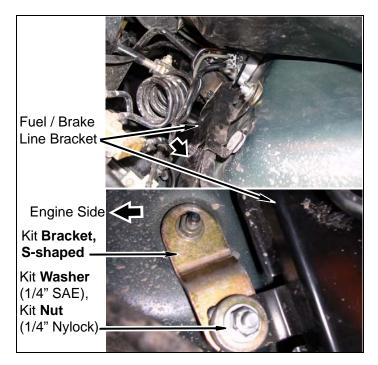
b. Install kit bracket, straight on the wheel well side of the fuel / brake line bracket with a kit washer (1/4" SAE) and kit nut (1/4" nylock) as shown. Install two kit brackets and fuel / brake line bracket on firewall with two nuts.
