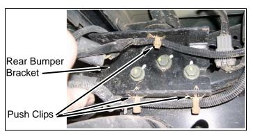
c. Disconnect two wiring harness connectors from wiring harness.
