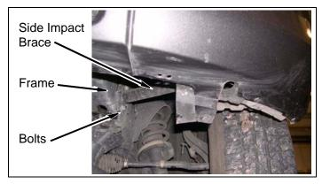
i. Remove four bolts and skid plate from frame and vehicle.
