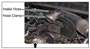
b. Install two clips, hose clamp, axle vent hose, and axle vent hose clip on air cleaner base.
