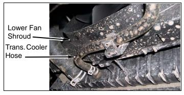
c. Install hose clip, metal transmission cooler hose, and transmission cooler hose on fan shroud and lower fan shroud.
