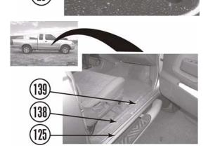
b. Remove three screws (140) and two kick plates (141) from cab (125).
