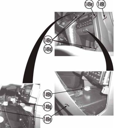
e. Remove six screws (149i) from storage console (149b) and cab (125).
