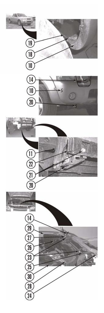
c. Remove bolt with captive washer (31) from air cleaner housing top (30).
