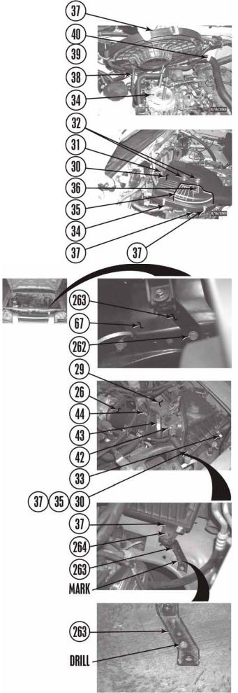
f. Install bracket (263) on lower air cleaner housing (37) and driver side wheel well (67) with two bolts with captive washers (262 and 264) as shown.
