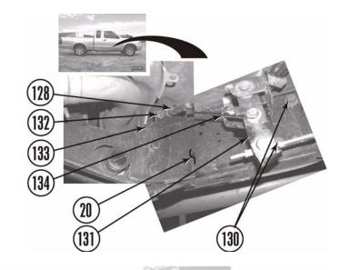
d. Remove nut (135), clamp (136), and parking brake housing (128) from cab stud (137). Pull cable housing to gain 1/2" of length.
