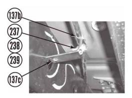
b. Install *kit* bracket (137c) on frame (20) driver side with bolt (137a).
