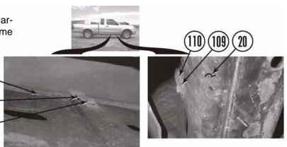
d. Remove clip (111) from two brake lines (112) passenger side wheel well (67).
