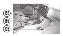
f. Remove five screws (158), 4wd intermediate shift boot (159), 4wd inner shift boot (160), from cab (125) and 4wd shift lever assembly (149).
