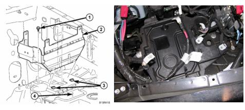
11. Remove the three nuts (1) securing the battery tray (2) to left inner fender (3). Lift the battery tray (2) out of the engine compartment and remove from the vehicle.
