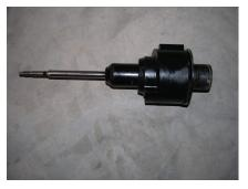
28. Install the boot over the strut and with one of the replacement washers, pull the boot over the washer at the top of the strut and zip tie the boot to the bottom of strut.
