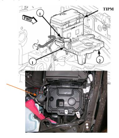
7. Using a appropriate flat bladed tool, depress the four mounting clips (3) to disengage and remove the TIPM housing (1) from the TIPM bracket (2) mounting tabs.
