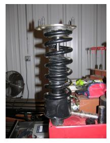
31. Reinstall the strut assembly into the vehicle and start the upper nuts, hand tighten only. Reinstall the lower strut clevis and hand tighten the bolt at the strut. Install the lower clevis bolt into the lower control arm
