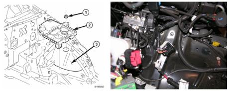
12. Remove the axle vent tube and ground wire from the 2 strut studs.
