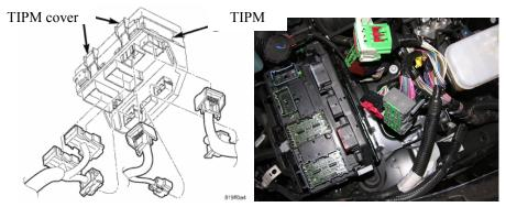
9. Remove the TIPM and put it in a safe place.
