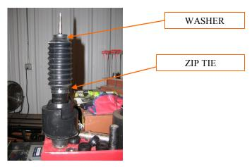
29. Press out the stock upper strut plate studs and press them into the lift strut plate. Note that the plate matches what strut that you are working on. There are LT and RT side plates.
