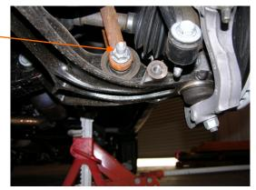
20. Remove the upper control arm ball joint nut with a 21mm wrench and separate the upper ball joint from the knuckle.
