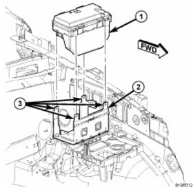
8. Disconnect each of the seven TIPM wire harness connectors from the TIPM housing. NOTE: Take care when removing the connectors.
