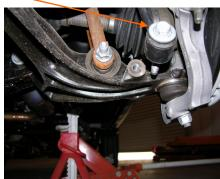
19. Remove the lower bolt at the lower control arm securing the clevis bracket with a 24mm socket.
