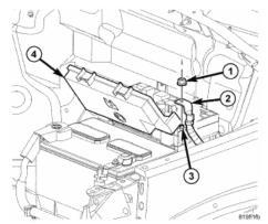
6. Disconnect the purge solenoid (1) from the battery tray (2) by pulling up on the solenoid and push away from the tray.
