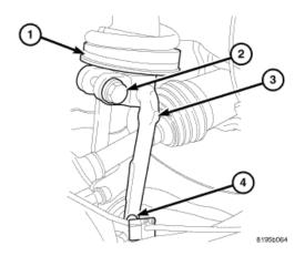
23. Remove the 4 upper strut nuts and remove the strut from the vehicle.
