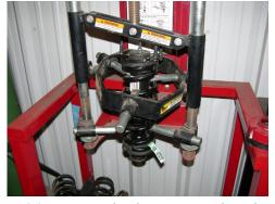
26. Remove the dust cover and washer from strut shaft.
