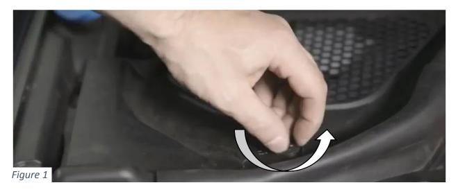
2.4 To remove the reinforcement braces (only one shown in picture, there are 2 on the car) use an inverted Torx E14 on the top bolts and a 16mm socket wrench on the bottom bolts.
