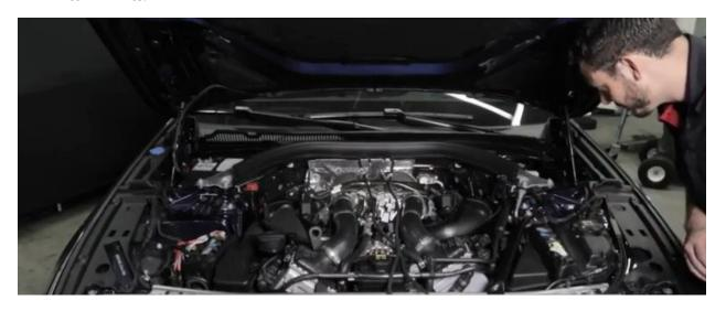
2.5 To remove the snorkels (highlighted), simply pull towards the rear of the vehicle, releasing it from the front clips. Once you've removed the rear hose clamps holding the snorkels in place, simply remove it from the engine bay.
