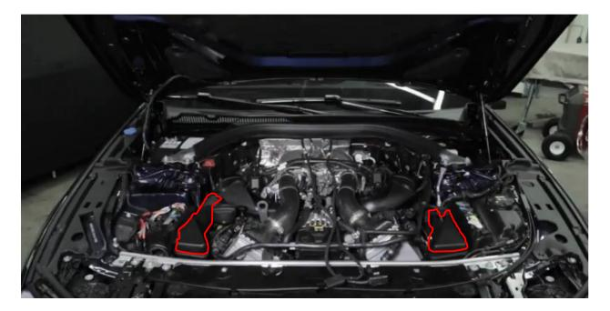
3. Examine the DINANTronics Elite harness supplied with this kit. There are two legs to this harness, which are identical to each other. The DINANTronics Elite attaches to 2 MAP sensors that are located below and in front of the engine (see figures 2-4)
