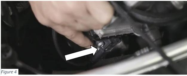
4. Study the locking system on the DINANTronics Elite connectors until you are familiar with how the two connector halves are released. Some locks will require the use of a small flat blade screwdriver to release the tang.
