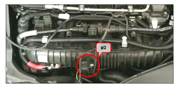
10. Like the previous sensor, install the DINANTronics harness in between the manifold pressure sensor and the factory wiring harness. The connectors are unique, and can only be installed one way. Make sure that the locking tangs on both connections are secure. II. Route the DINANTronics harness to sensor #3, located at the end of the fuel rail.
