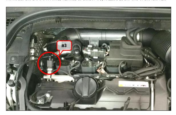
12. The fuel rail pressure sensor connection could be one of two configurations. Please examine your harness connector and compare it to the photos below. One style is a D-shape, while the other style is an oval-shape. If you do not have the correct harness for your vehicle, please contact Dinan for an exchange -- do not continue with installation
