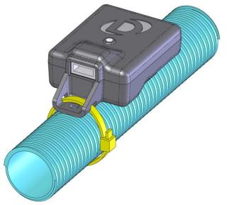
9. Mount the module at the location shown below. Also use a zip-tie to secure the connector and excess harness to the plastic tube running directly underneath. Also ensure adequate slack in the wiring harness to allow for engine movement.
