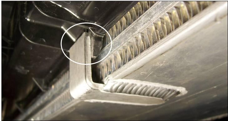
9. When you have the Intercooler opening sufficiently clearanced you will need to install the hose coupler latches from the stock intercooler onto the Dinan intercooler. Check the condition of the O-Rings on the stock hose's and replace if needed.
