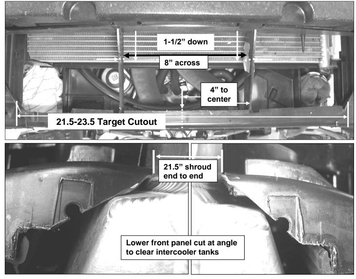
11. Use the Dinan Intercooler to check fit your trimming efforts. Lift the Intercooler into place while guiding the hoses into the Intercooler tubes. It is important to latch the bent tangs on the lower back edge of the Intercooler onto the two tabs of the radiator shroud. See below.
