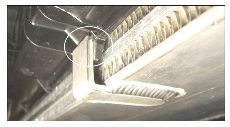
12. When you have the Intercooler opening sufficiently clearanced you will need to install the hose coupler latches from the stock intercooler onto the Dinan intercooler. Check the condition of the O-Rings on the stock hose's and replace if needed.
