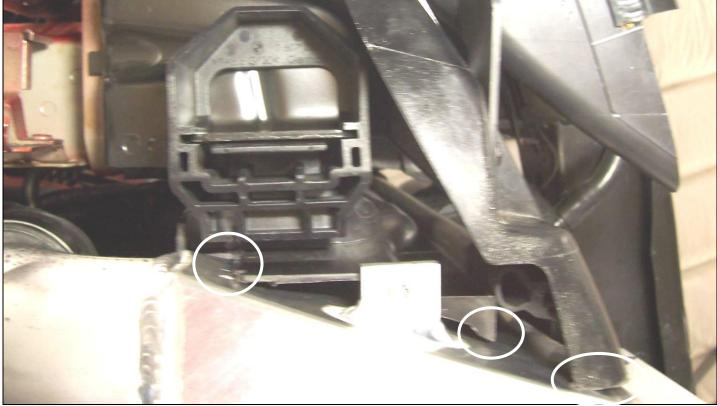
8. The two photos above show where the Intercooler tanks meet the areas to be trimmed. You may be able to trim less than the photo shows, as this was the prototype car install. I purposely overexposed the photo so the "hard to see" black plastic is much more visible. I have circled the areas of contact that require trimming. Intercooler opening will actually need to get larger as you
