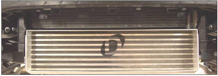
7. Observe the next two photos showing the bottom view of each end of the installed Intercooler before you cut out the opening. See where the two mounting screws are for the Intercooler. You want to be careful to not cut out the two mounting screw holes.
