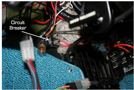
Figure 2 - Locate Circuit Breaker
