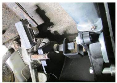
Figure 5 - Install Motor Assembly
