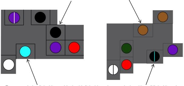
Remove existing light blue or black with light blue wire terminal and install light blue wire terminal from new harness
