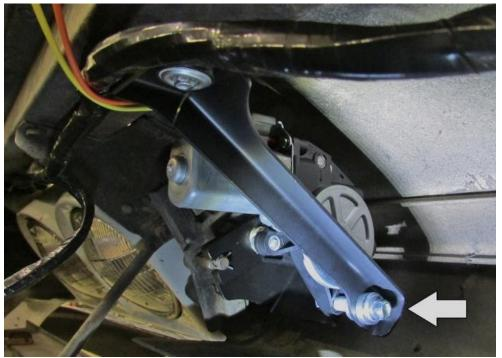
Figure 6 - Tighten Support Bracket
