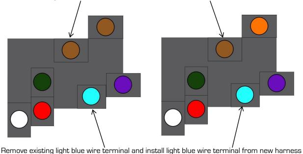
Figure 9 – End View (Harness Side) Late 1965 to 1966 Corvette
