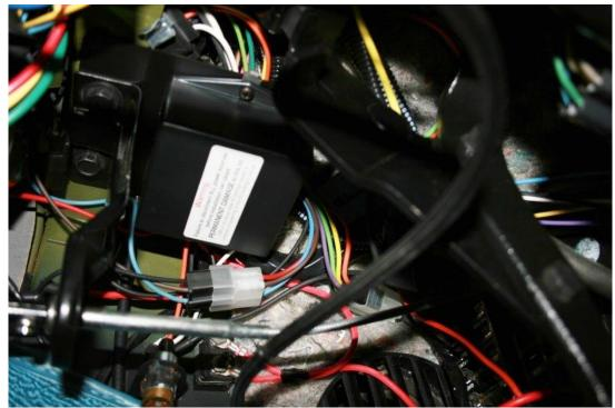
Figure 14 - Mount Control Module
