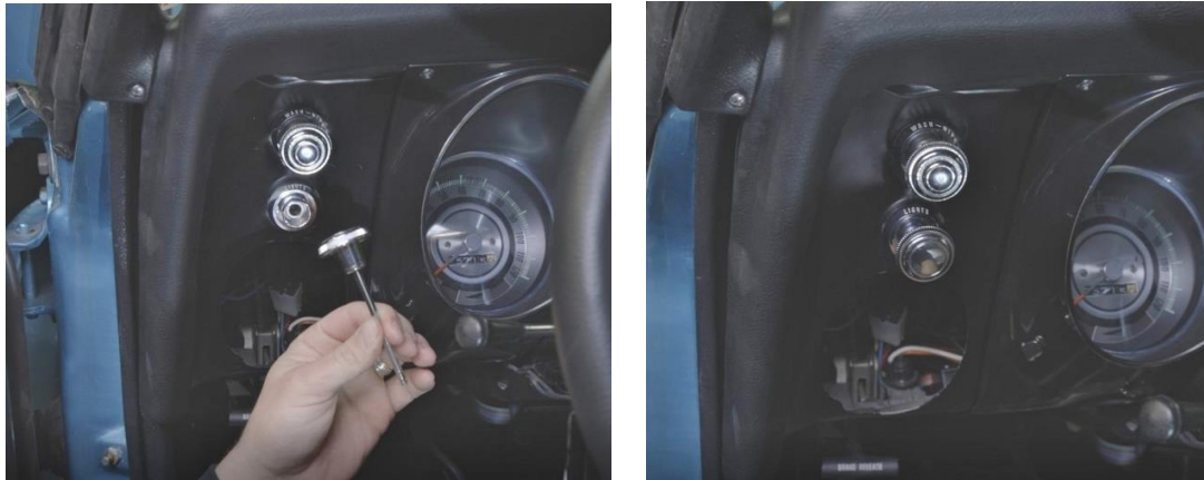
Figure 39 – Re-install Headlight Knob
