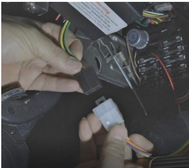
Figure 32 - Connect Harness to Module
