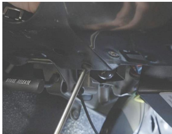
Figure 31 - Connect Ground Wire
