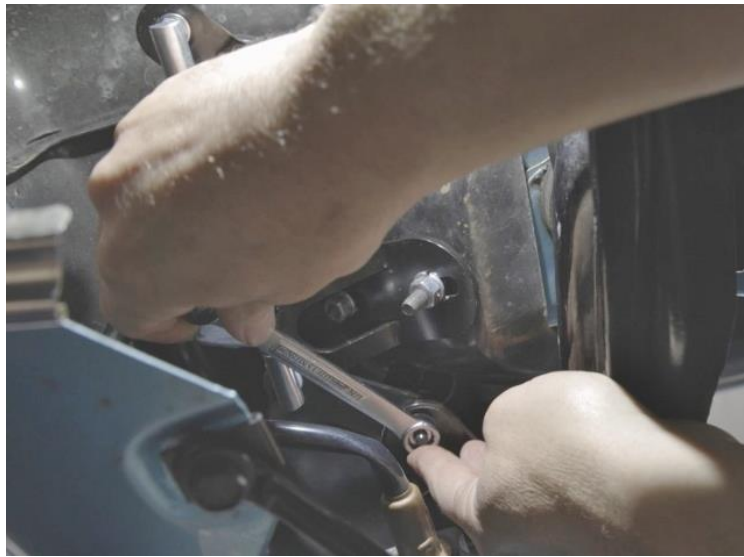
Figure 35 – Adjust Bell Crank Fastener
