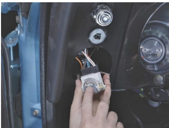
Figure 37 – Re-install Headlight Switch
