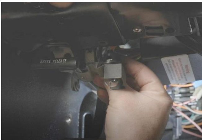
Figure 31 - Connect Ground Wire
