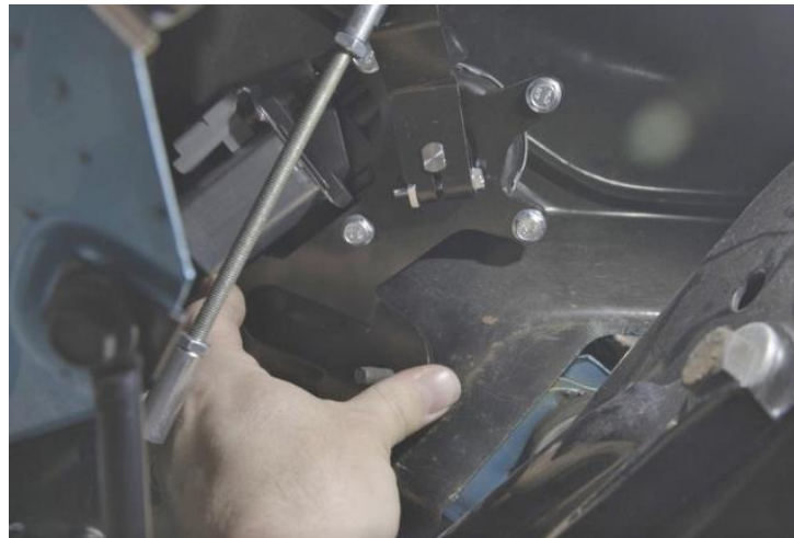
Figure 24 – Position Actuator & Bracket Assembly
