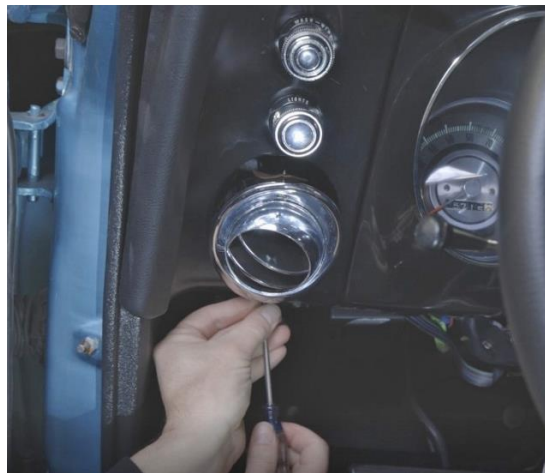
Figure 40 – Re-install Astro vent
