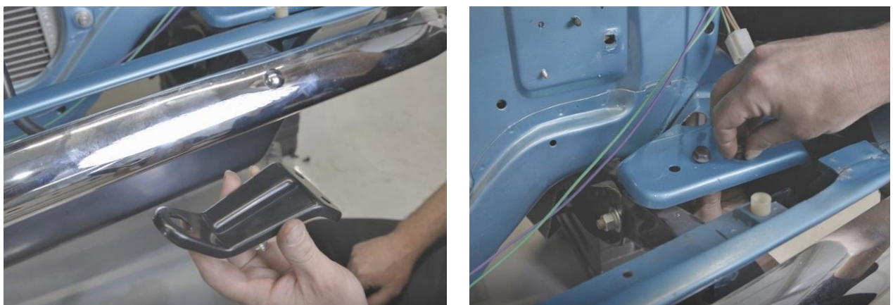
Figure 17 – Install Bell Crank Support Bracket
