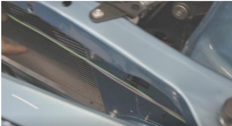
Figure 14 - Route Passenger Side Harness
