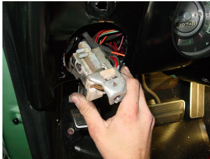
Figure 6 - Accessing the Headlamp Switch
