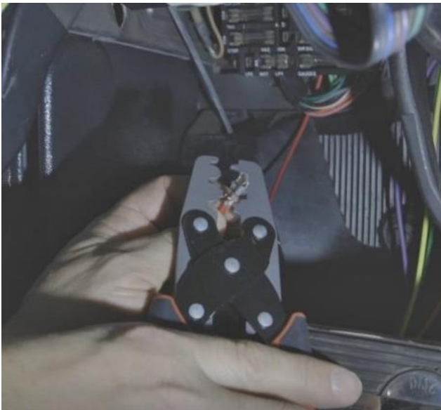
Figure 29 – Crimp Terminal to Red Wire
