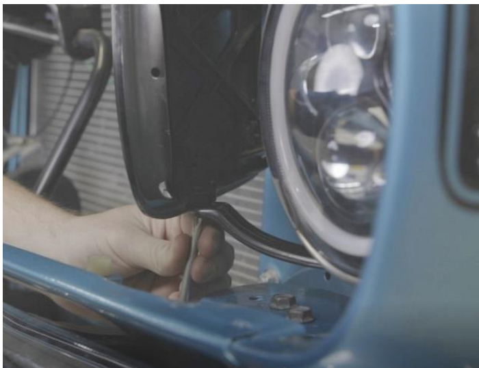
Figure 21 - Attach Bell Crank
