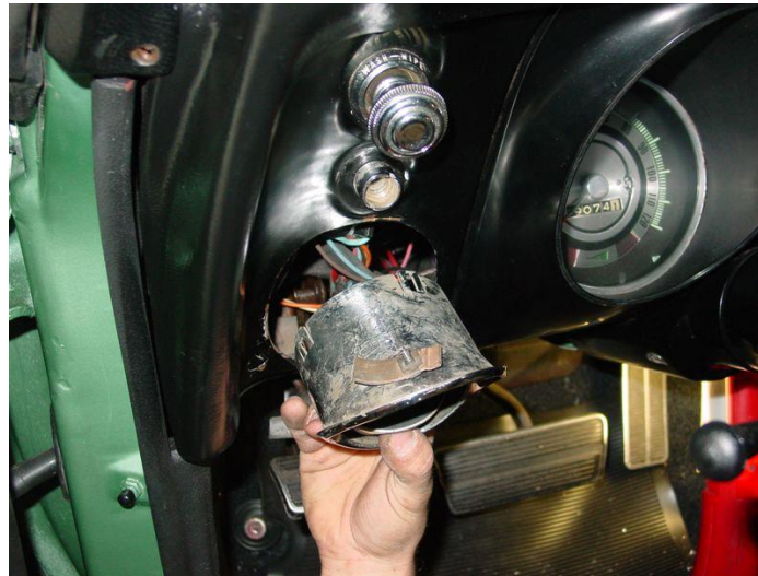
Figure 5 - Removing the Astro Vent
