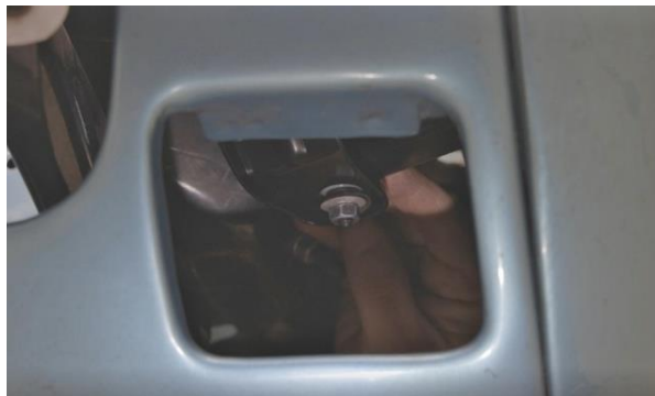
Figure 19 - Install Bell Crank Fasteners
