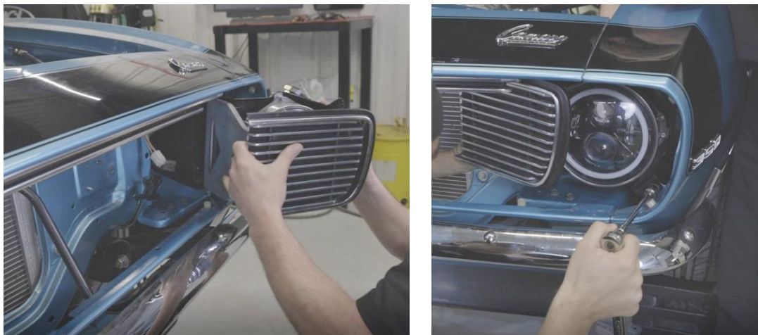
Figure 20 - Re-install Headlight Door Assembly
