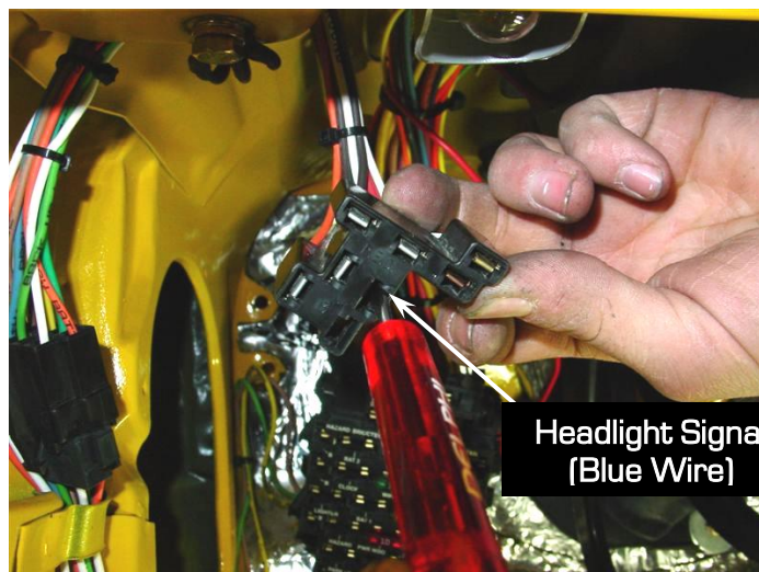
Figure 7 - Locating the Blue Wire
