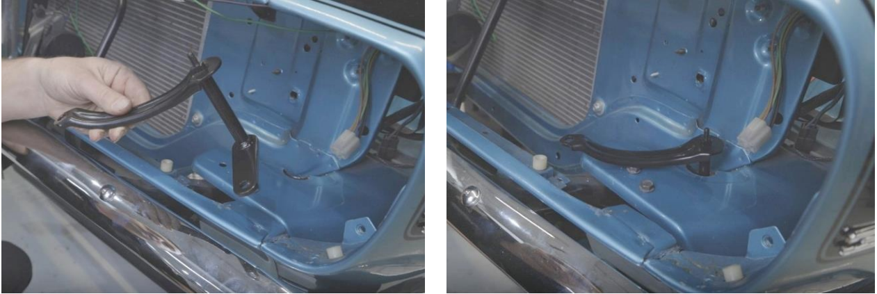
Figure 18 - Position Bell Crank
