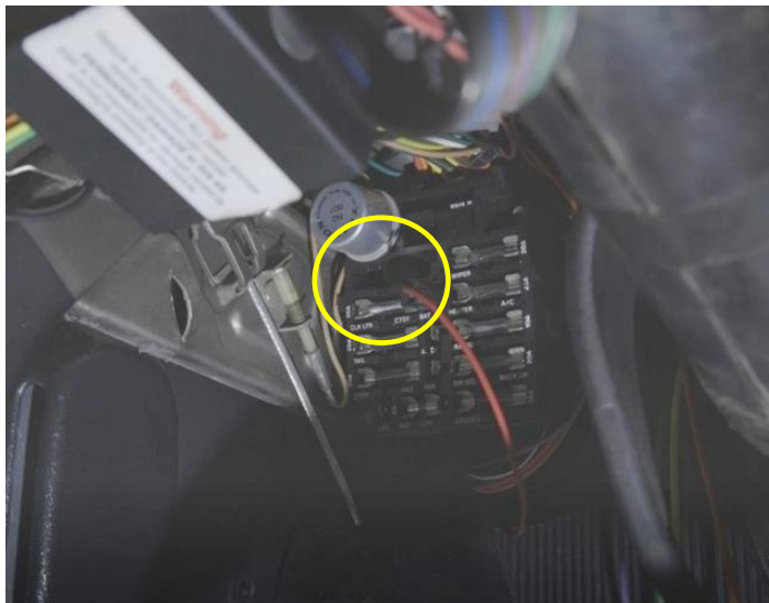
Figure 30 - Attach 12V Constant Power Source
