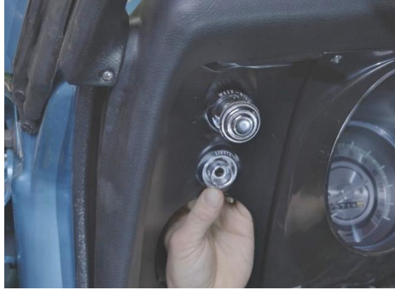
Figure 38 – Re-install Headlight Bexel and Switch Nut
