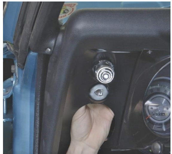
Figure 37 – Re-install Headlight Switch
