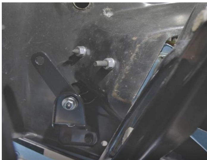
Figure 22 - Remove Core Support Fasteners
