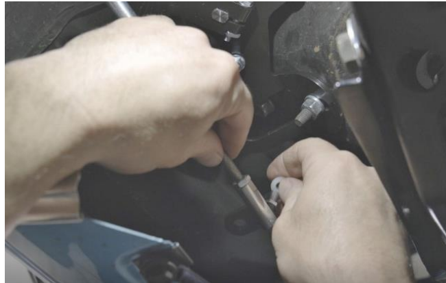
Figure 26 – Install Nylon Bushing
