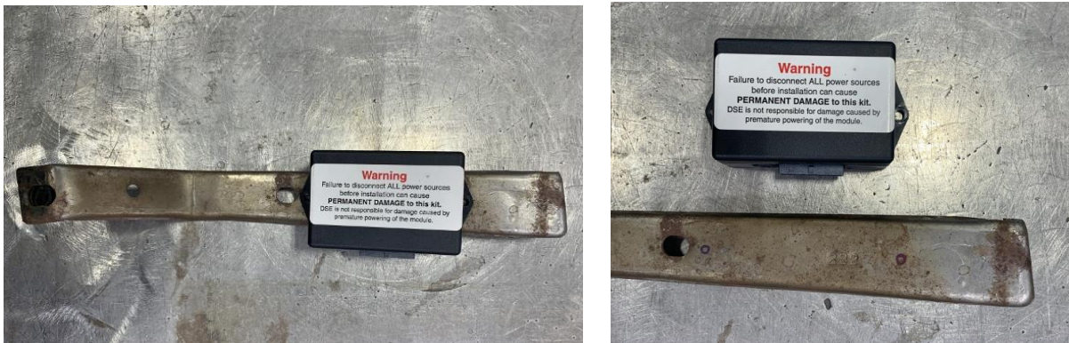
Figure 19 – Position the Wiper Control Module
