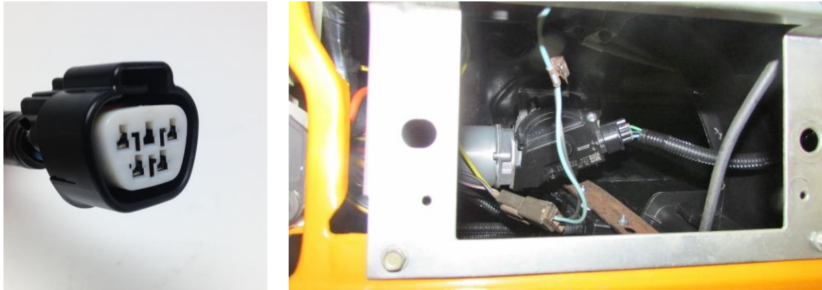
Figure 18 – Wiper Motor Connector
