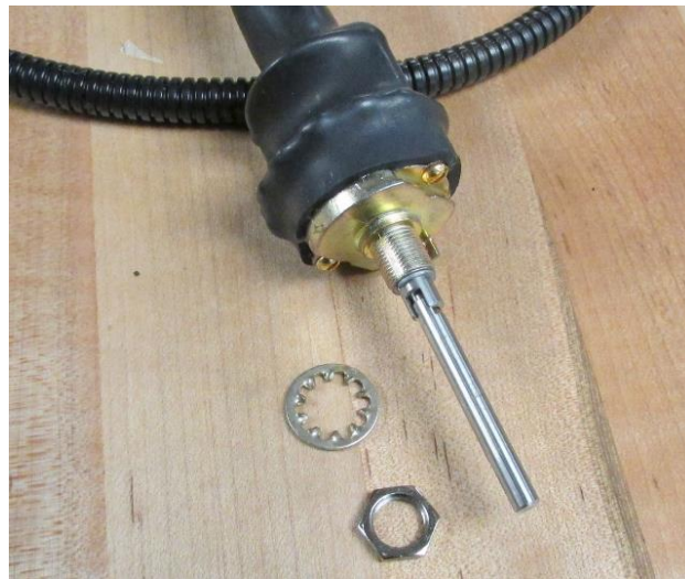
Figure 5 - Remove Nut & Washer
