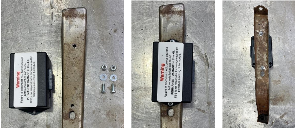
Figure 20 – Mount the Control Module
