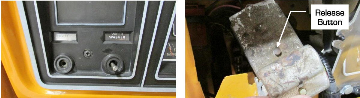
Figure 1 – Remove Wiper & Headlight Knob
