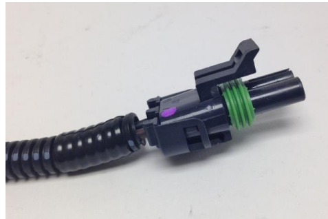
Figure 22 – Washer Pump Connection
