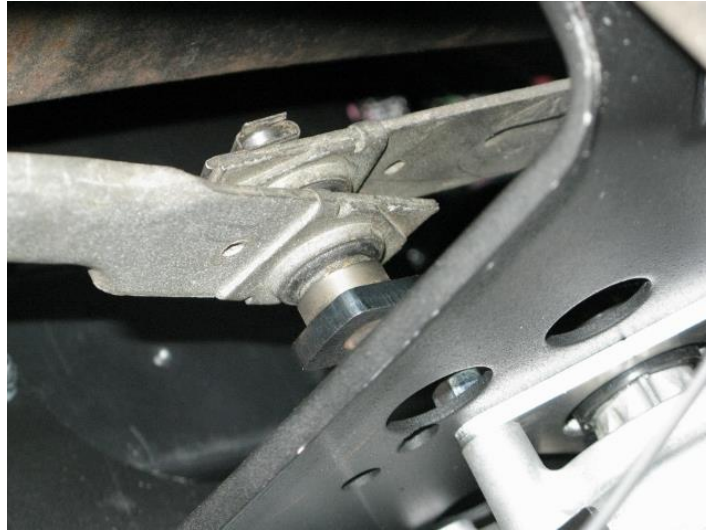
Figure 17 – Attach Wiper Linkage to Pitman Arm
