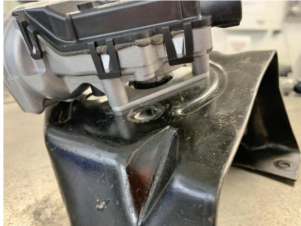
Figure 14 - Drill Motor Mount Holes
