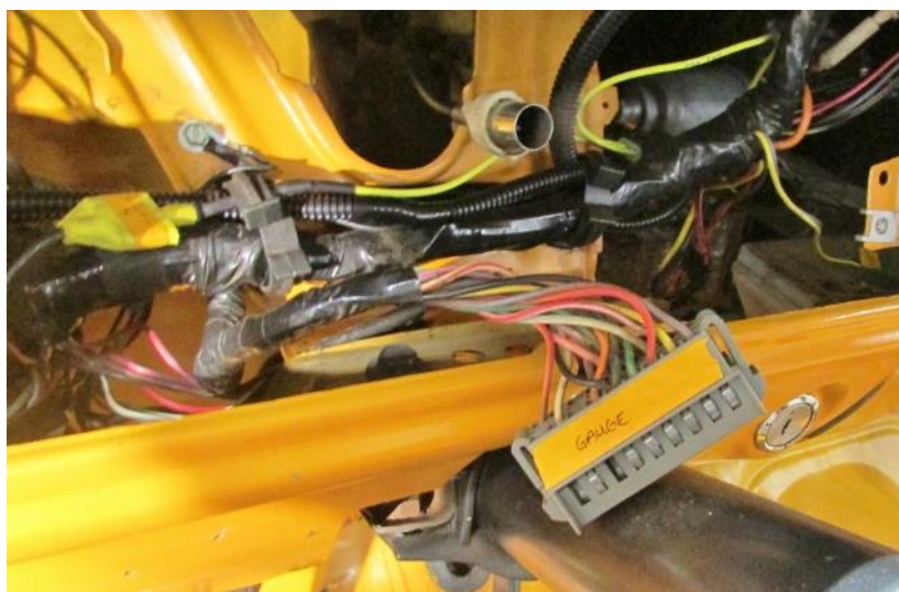
Figure 3 – Remove Gauge Cluster
