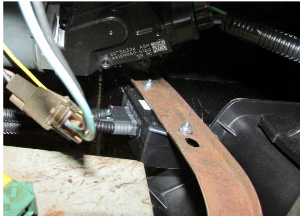
Figure 21 – Install Dash Support Bracket with Module
