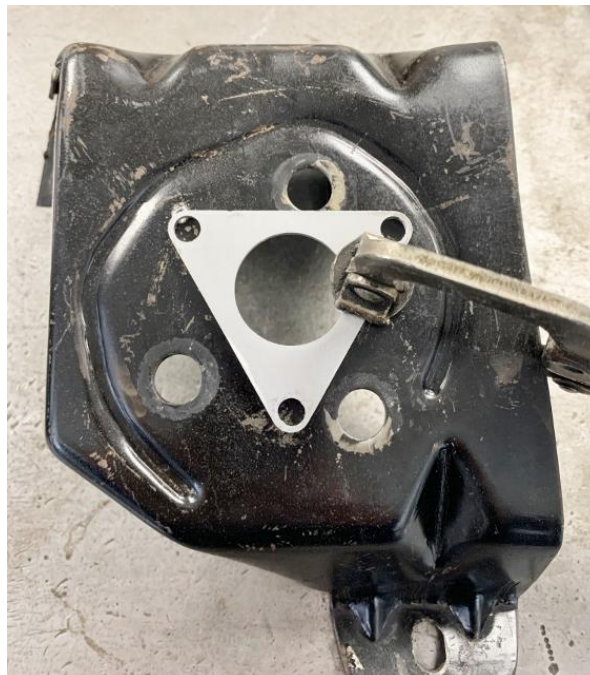
Figure 11 – Wiper Motor Spacer
