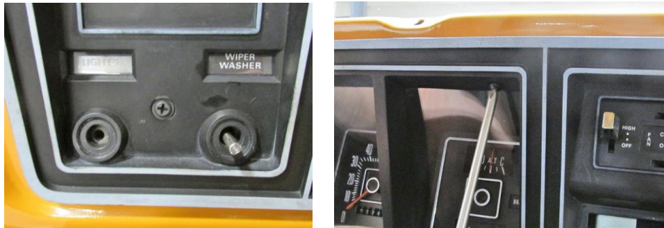
Figure 24 - Re-Install Gauge Bezel
