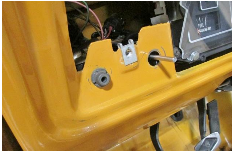
Figure 7 - Install DSE Switch & Bracket
