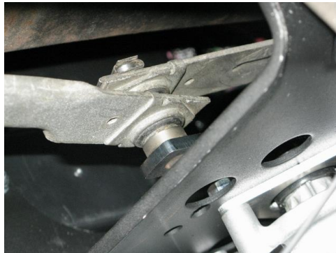
Figure 9 - Attach Wiper Linkage to Pitman Arm
