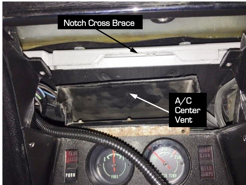
Figure 12 - 1968-69 C3 Cross Brace
