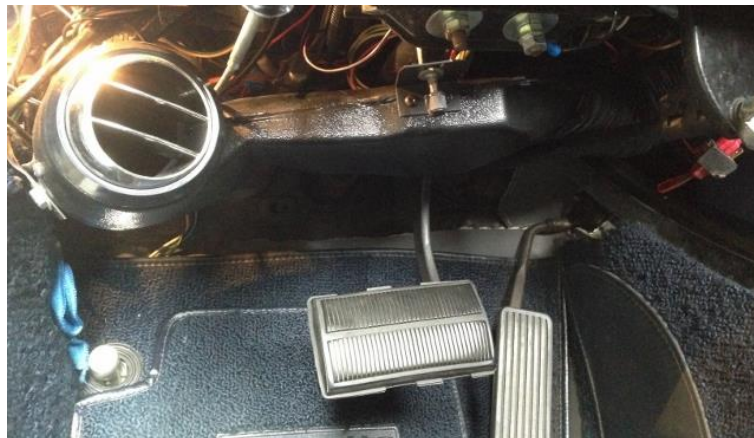
Figure 10 – Remove A/C Duct
