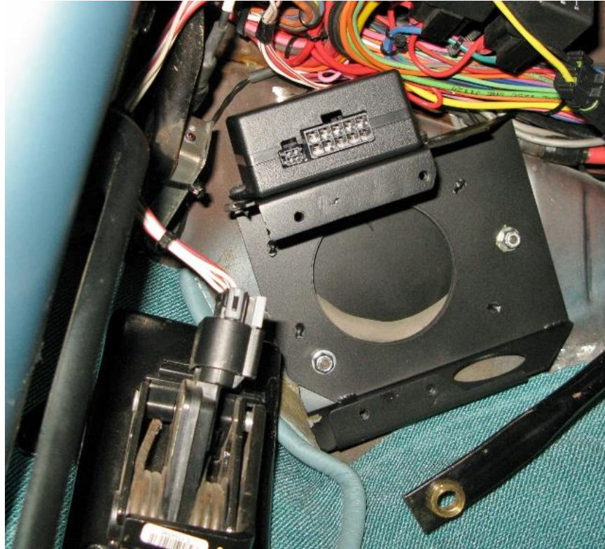
Figure 5 - Install Wiper Control Module
