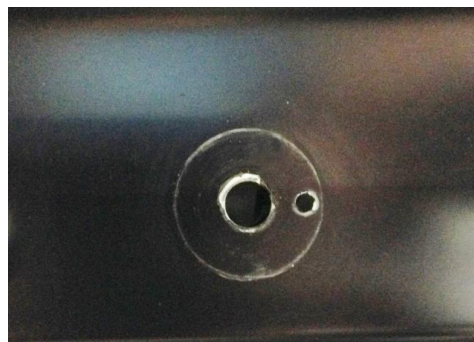
Figure 10 - Drill Anti-Rotation Hole
