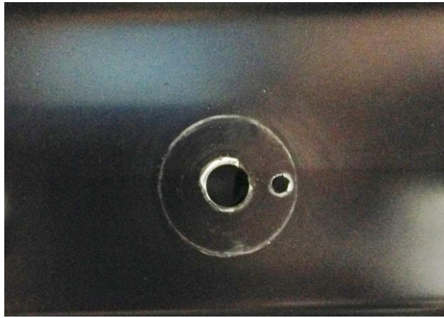
Figure 5 - Drill Anti-Rotation Hole
