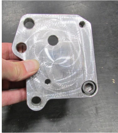
Figure 6 - Install Socket Head Bolt & Spacer
