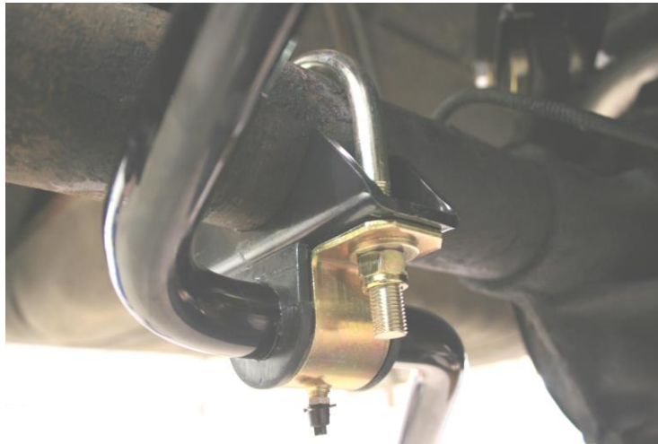
Figure 4 – Anti-Roll Bar Mounted on Rear Axle
