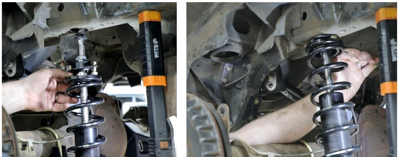
Figure 39 - Install Shock & Spring Assembly
