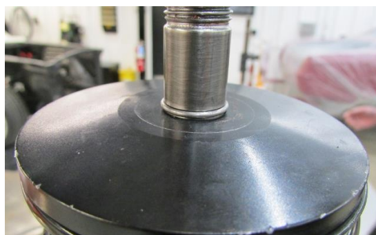
Figure 35 - Install Spring Perch & Retaining Ring
