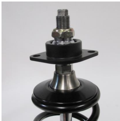
Figure 33 - Tighten Upper Shock Mount to Shock
