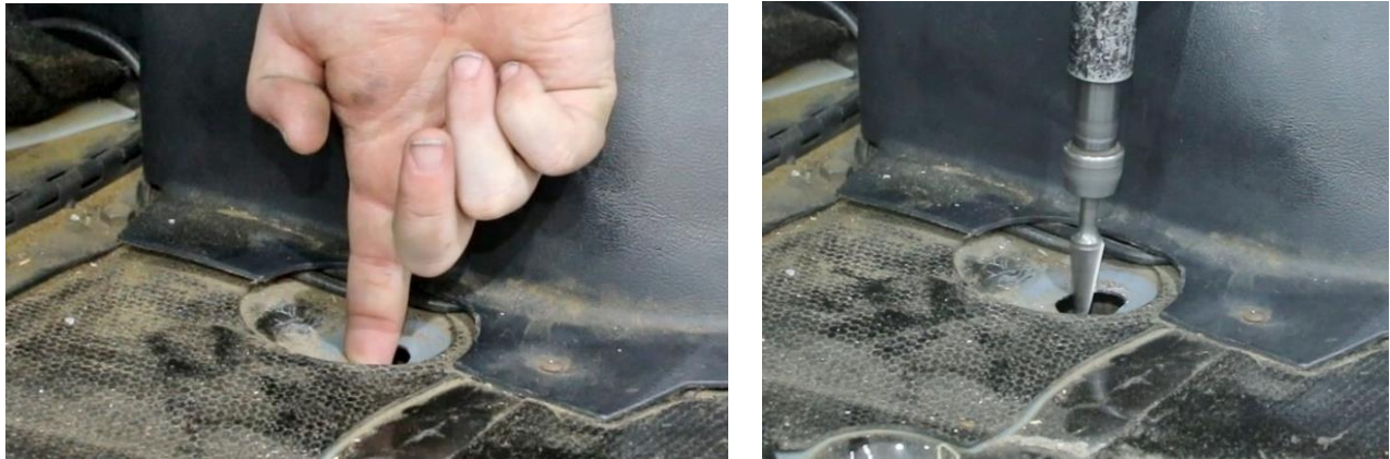
Figure 6 - Locate Frame Rail
