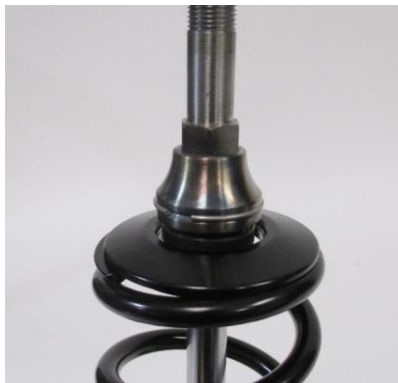
Figure 32 - Install Spring Perch & Retaining Ring
