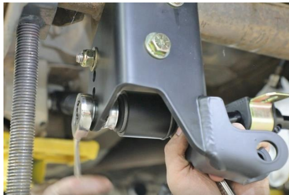
Figure 21 – Install Lower Trailing Link
