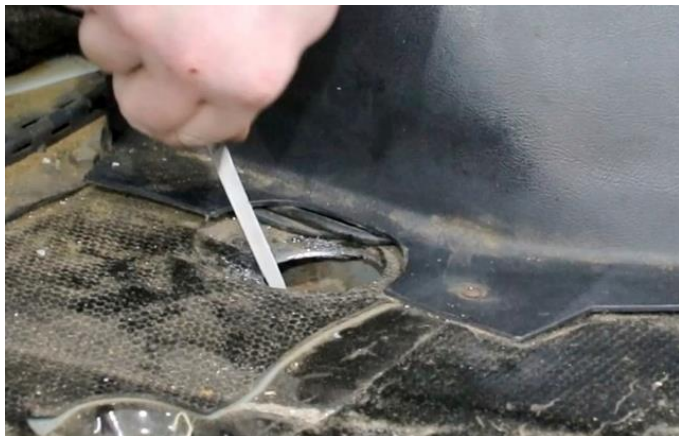
Figure 9 - Install Button Plug
