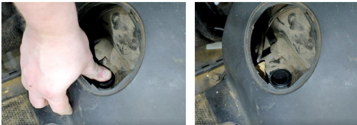
Figure 3 - Install Button Plug
