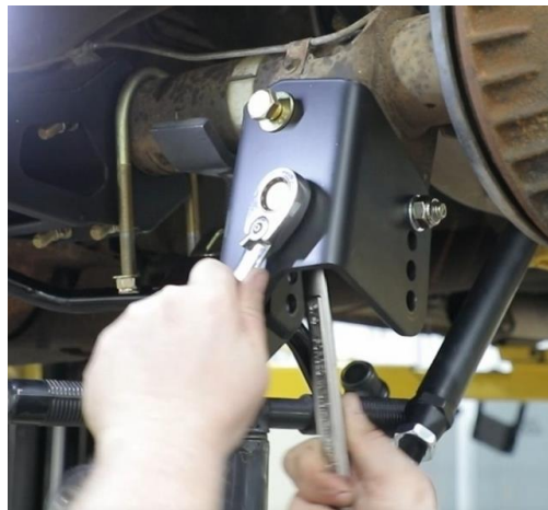
Figure 20 - Tighten Mounting Hardware
