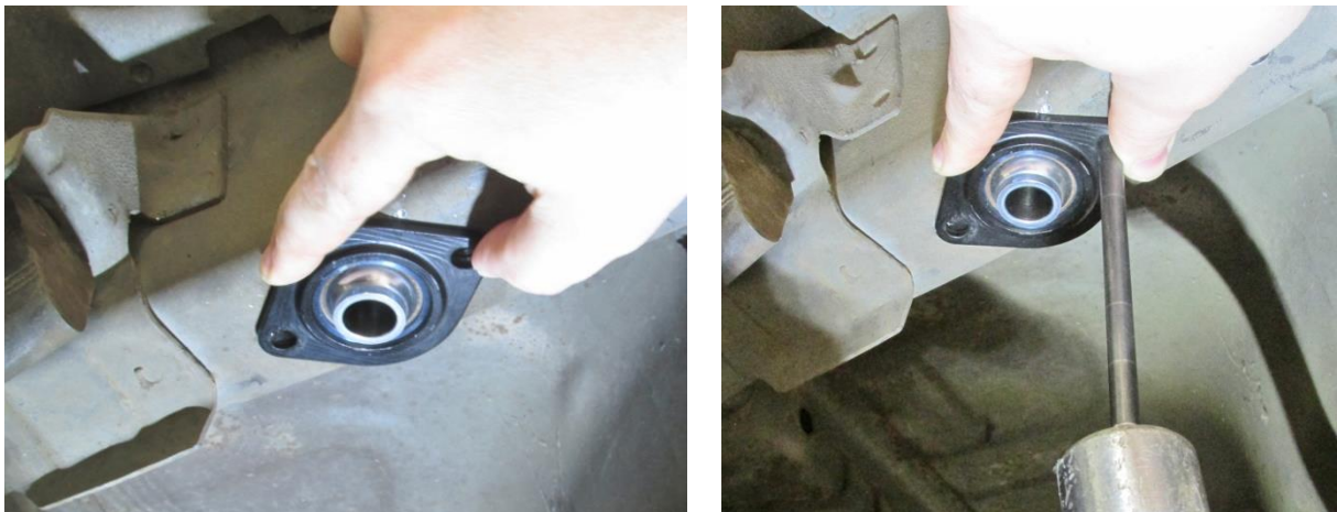
Figure 27 - Transfer Punch Shock Mount Locations
