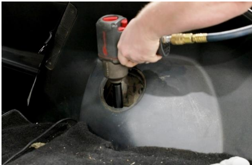
Figure 2 – Remove Upper Shock Nut
