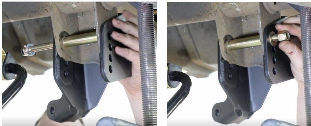
Figure 16 - Install Mounting Hardware
