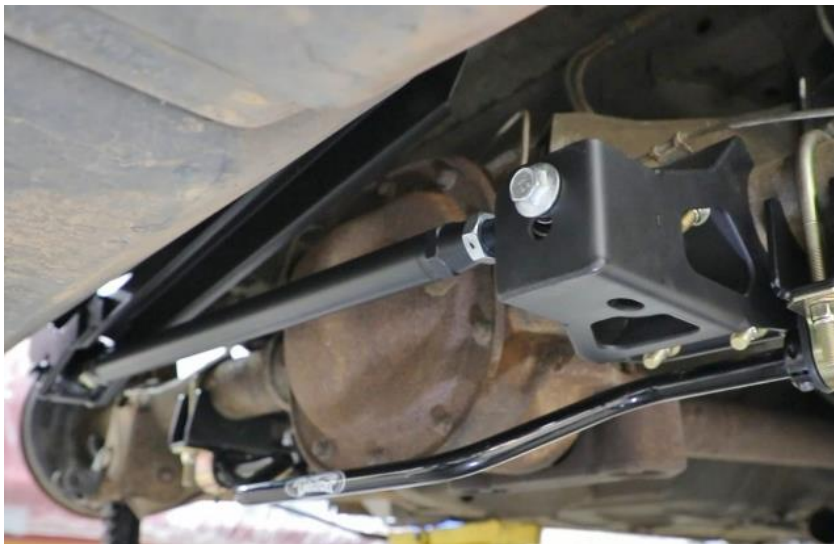
Figure 42 – Track Bar Installation
