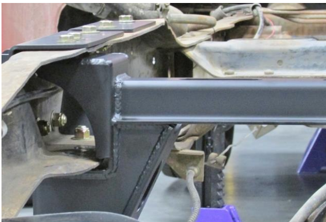
Figure 16 – Install Track Bar Crossmember
