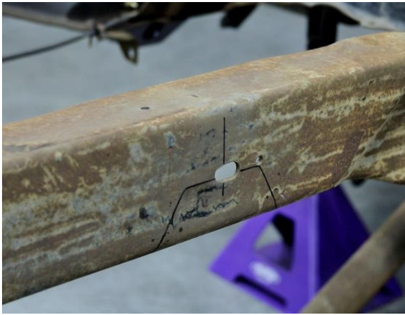
Figure 7 – Trace Frame Notch Cutout
