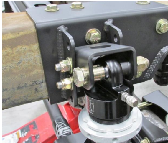
Figure 39 - Install Coilover Shock into Frame Mount
