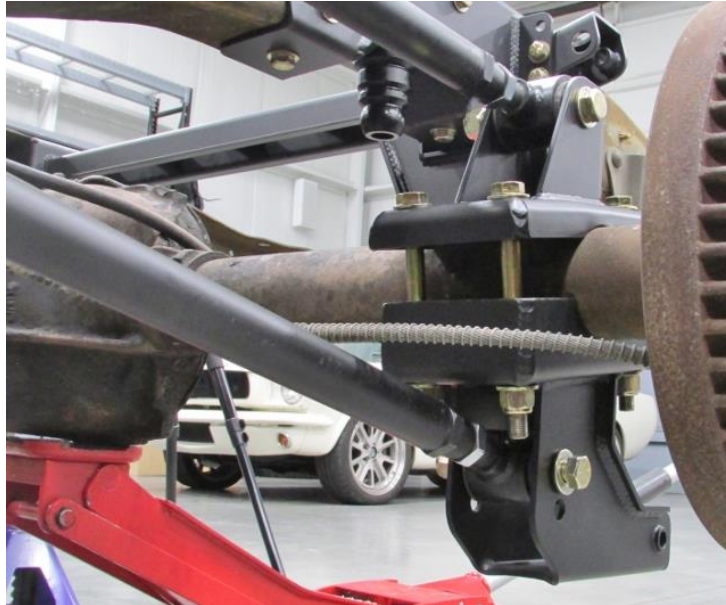
Figure 26 – Install Links to Axle Brackets (PN: 041750DS Shown)
