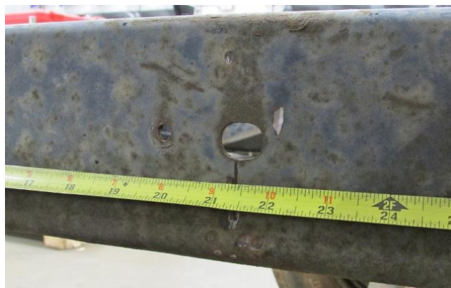
Figure 5 - Locate Notch Centerline
