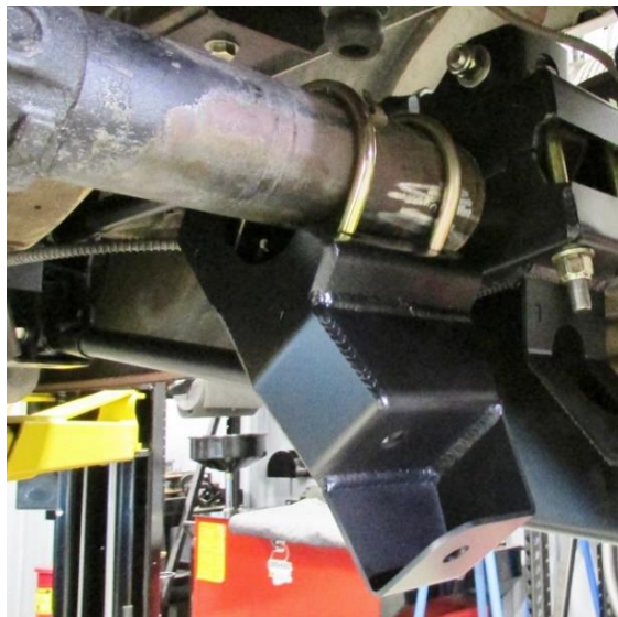
Figure 27 – Position Track Bar Axle Bracket
