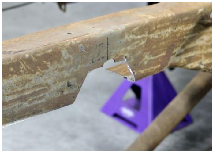
Figure 8 – Notch Frame Rail
