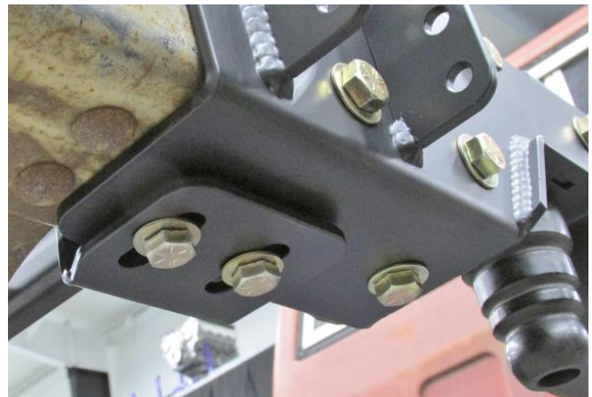
Figure 16 – Install Track Bar Crossmember
