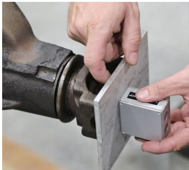
Figure 30 - Check Pinion Angle
