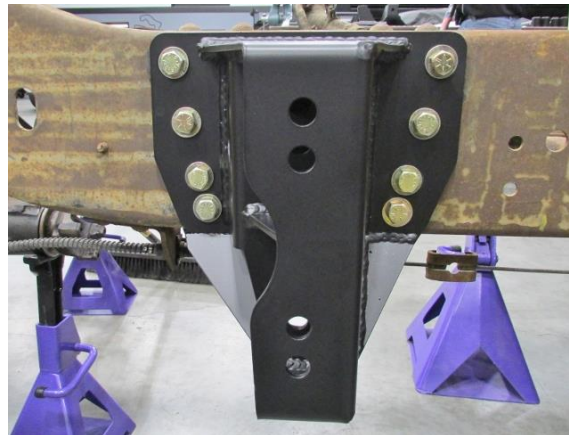
Figure 21 - Install Frame Bracket Assembly
