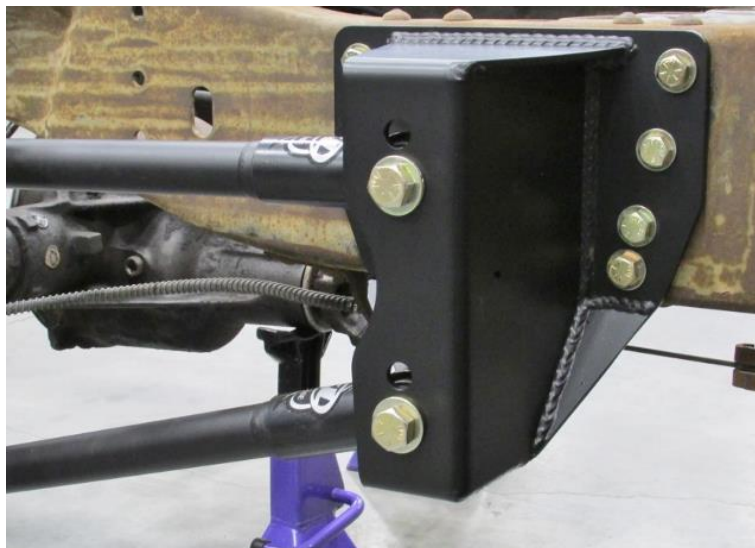
Figure 25 – Install Links into Frame Brackets
