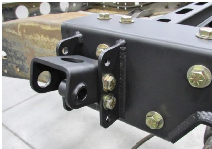
Figure 12 – Install Upper Shock Mounts (RH, Passenger Side)
