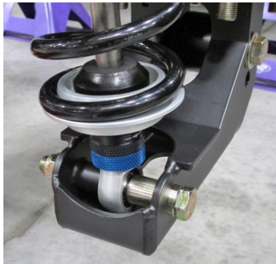
Figure 40 - Install Coilover Shock into Axle Bracket
