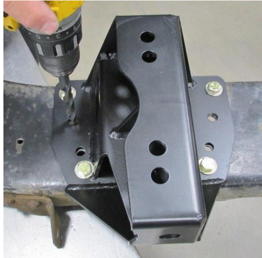
Figure 20 - Drill Mounting Holes
