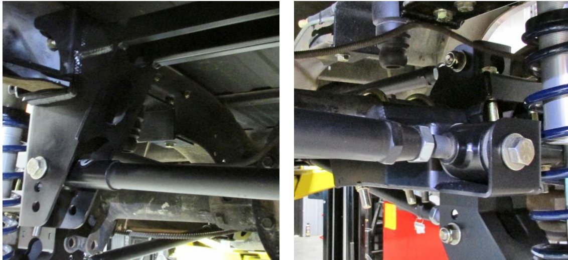
Figure 31 - Install Track Bar
