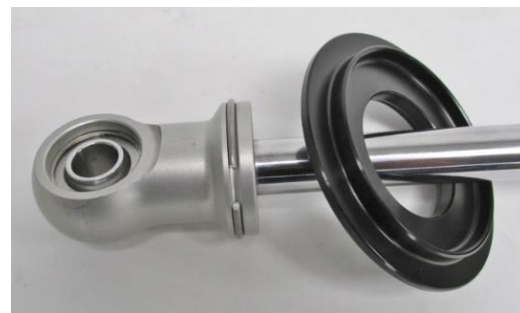
Figure 36 - Install Spring Perch
