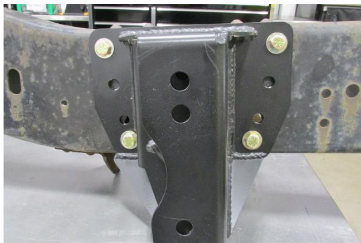
Figure 19 - Locate Mounting Holes
