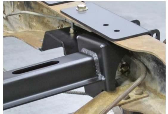
Figure 15 – Position Crossmember Assembly
