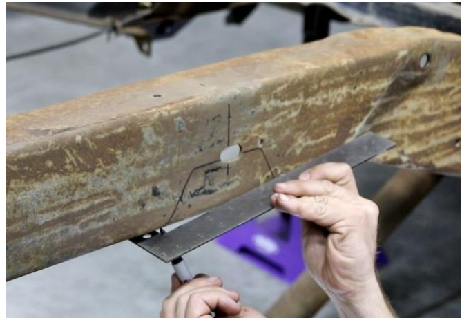
Figure 7 – Trace Frame Notch Cutout
