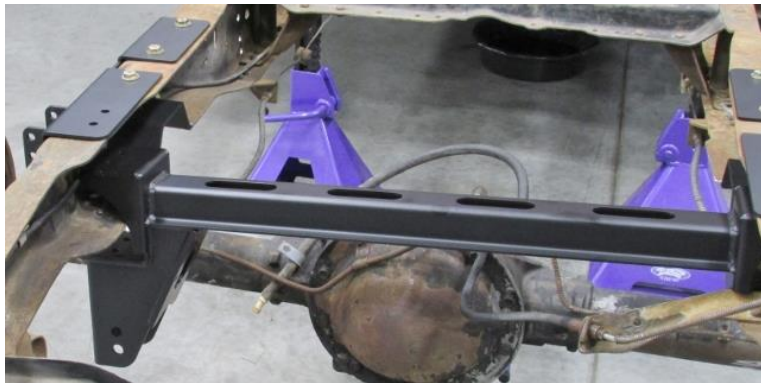
Figure 15 – Position Crossmember Assembly
