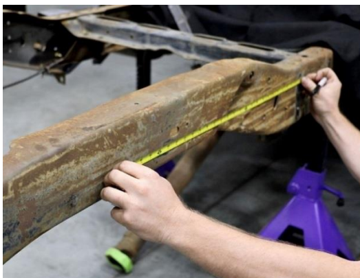
Figure 5 - Locate Notch Centerline
