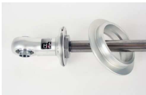
Figure 37 - Remove Upper Spring Seat
