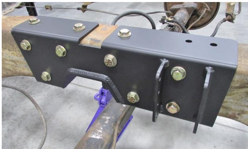
Figure 11 – Install Frame Notch Assemblies (LH, Driver Side)
