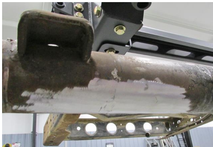
Figure 22 - Cut Off Factory Lower Shock Mount (Passenger Side)
