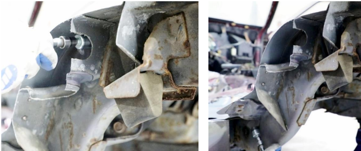
Figure 22 - Expose Spot Welds
