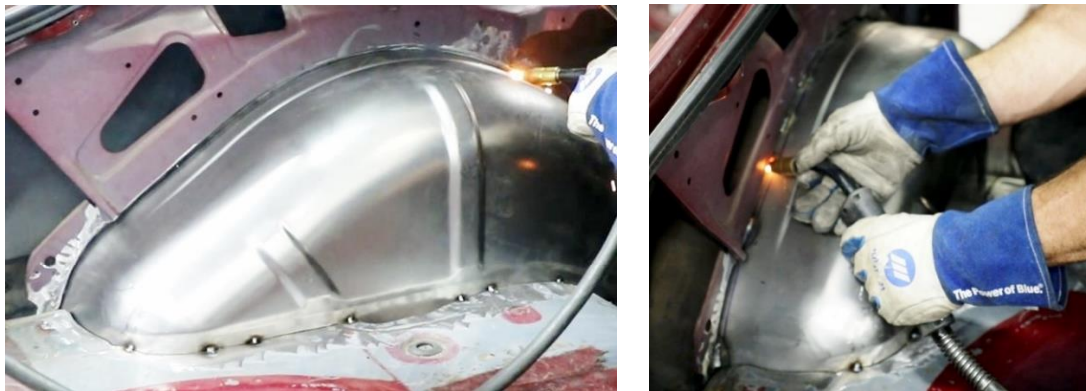
Figure 39 - Tack Weld Mini-Tub
