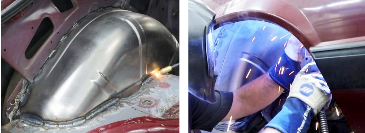
Figure 41 – Finish Weld around Mini-Tub
