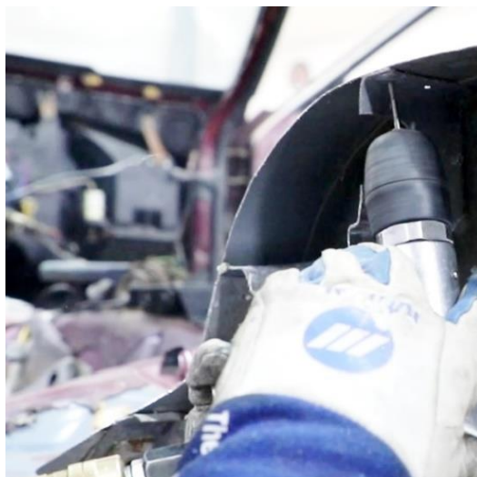
Figure 26 - Remove Spring Perch Spot Welds
