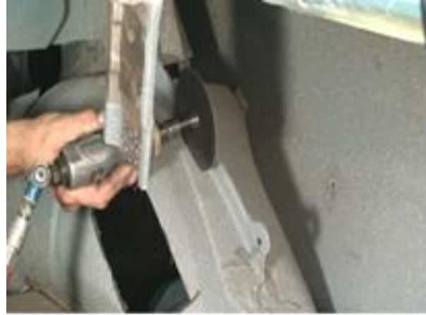
Figure 6b - Cutting the Factory Wheel Well
