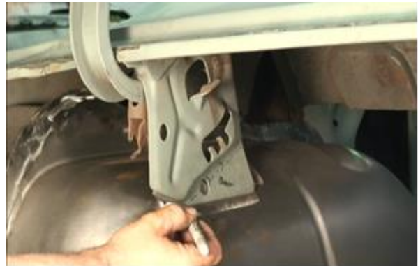
Figure 22b – Trimming Factory Brace & Flange
