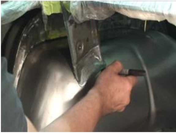
Figure 19a – Mark Driver Side for Welding
