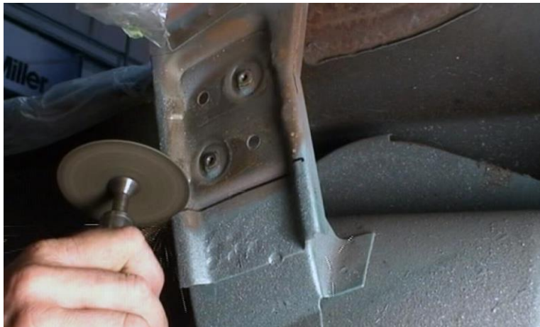
Figure 2 - Cutting the Driver Side Trunk Support Flange
