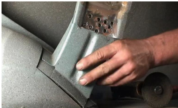
Figure 3 - Removing the Passenger Side Trunk Support Flange after Cutting
