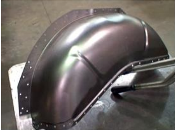
Figure 13b - Mini-Tub Ready to Weld
