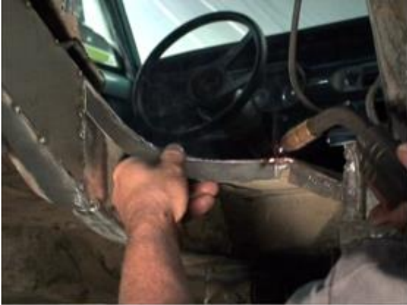
Figure 12a - Fabricate Front Flange
