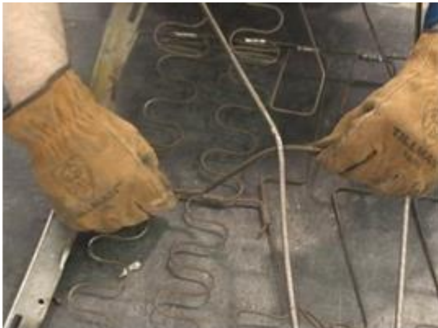
Figure 27 - Finished Flipped Cross Rod & Bent Diagonal
