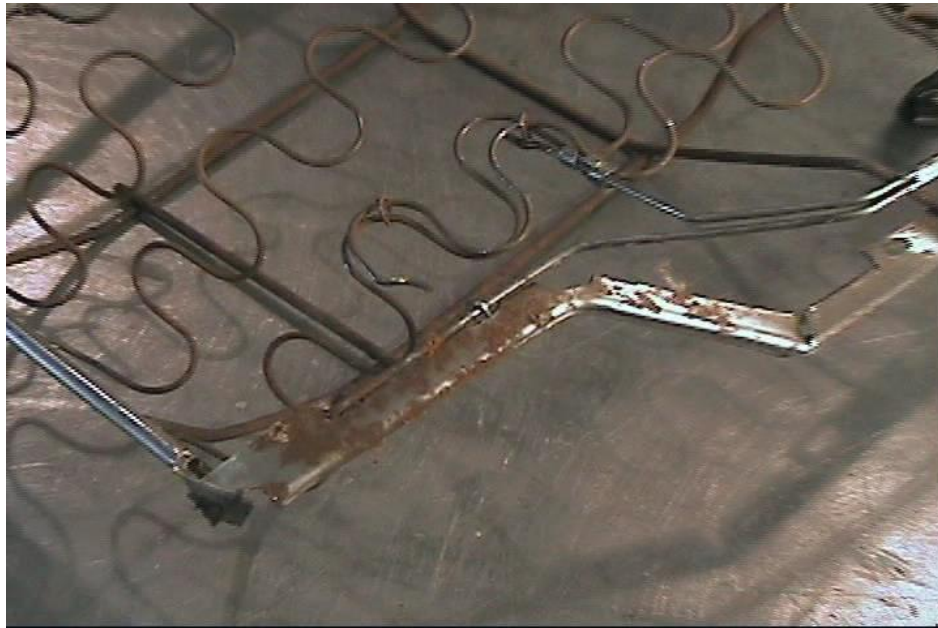
Figure 23 – Rear Seat Frame Modification
