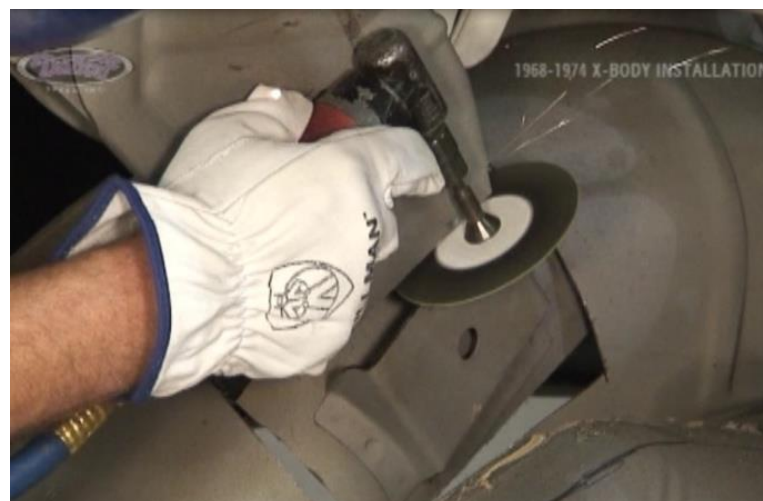
Figure 12 – Cut and Remove the Hinge Mount
