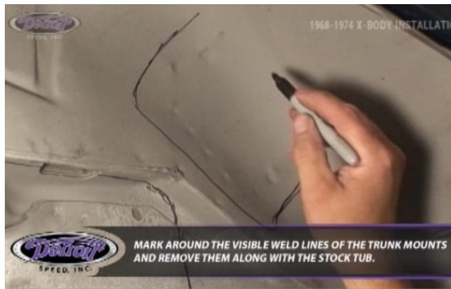
Figure 11 – Mark the Trunk Mounts
