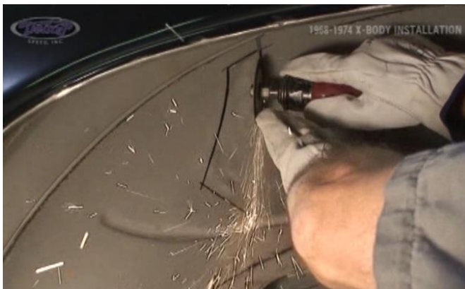
Figure 15 – Remove the Seat Brace
