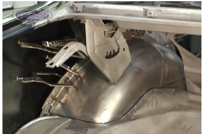
Figure 28 - Secure the Mini-Tub for Welding
