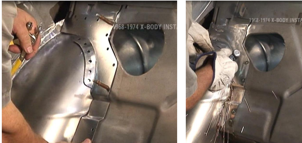
Figure 42 – Weld and Grind Seat Back Brace
