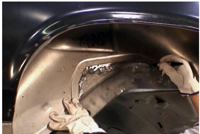
Figure 26 – Mark the Mini-Tub
