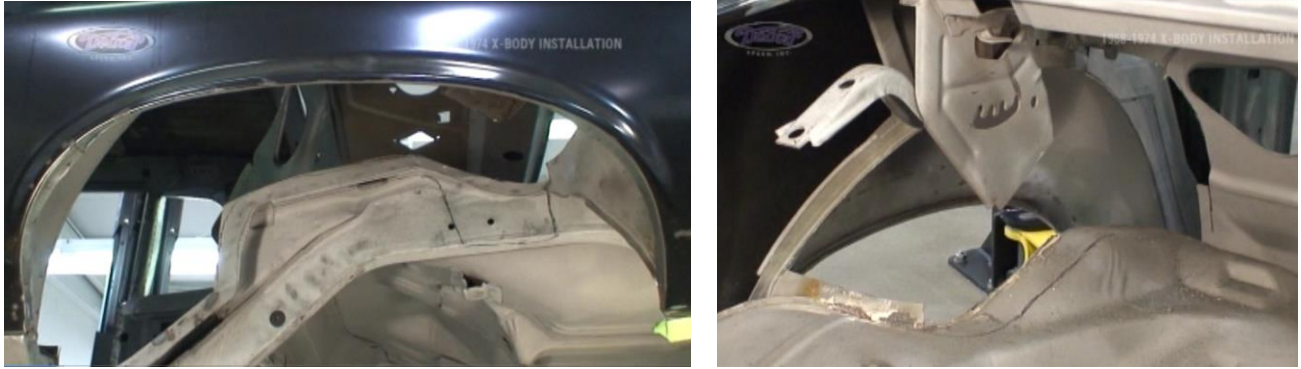
Figure 16 – Stock Inner Tub Removed
