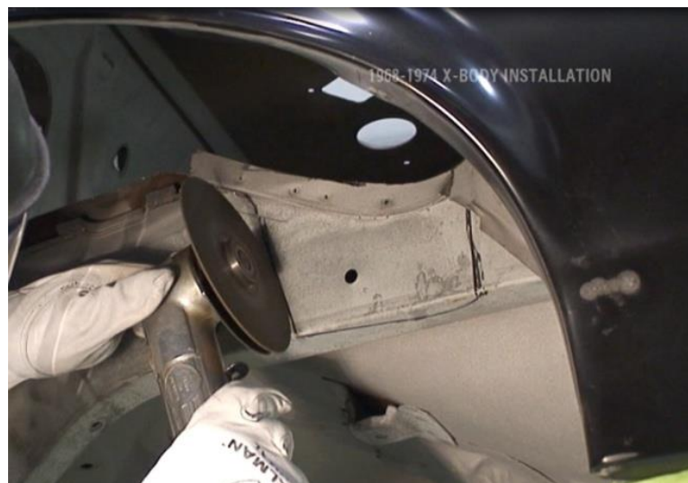
Figure 18 – Notch the Framerrail
