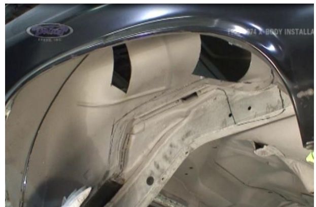
Figure 15 – Remove the Seat Brace
