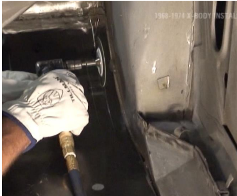
Figure 14 – Cut 1-1/4" Marked Lines
