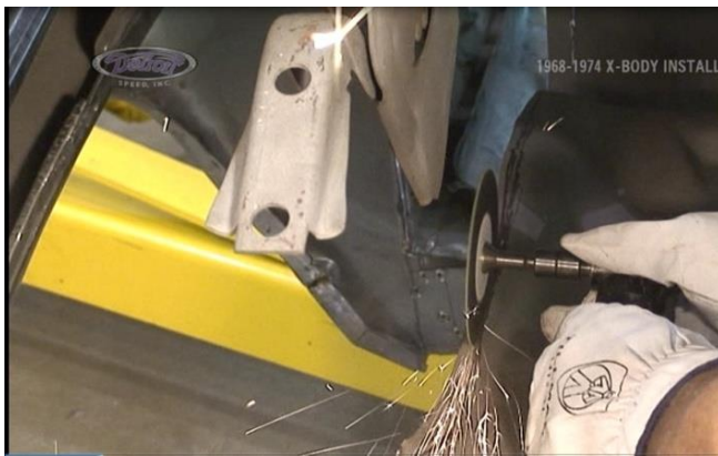
Figure 20 – Finish Cut and Grind Pre-Marked Lines
