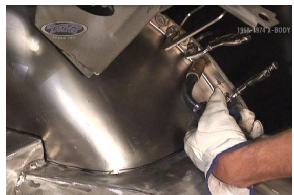
Figure 38 – Clamp and Weld to the Vehicle
