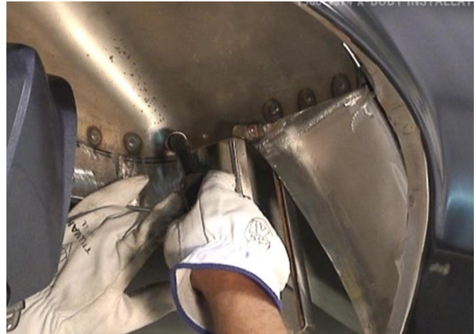
Figure 29 - Welding the Mini-Tub
