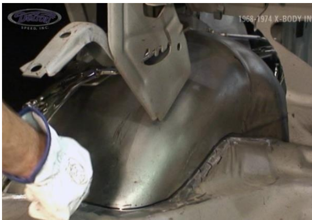
Figure 26 – Mark the Mini-Tub
