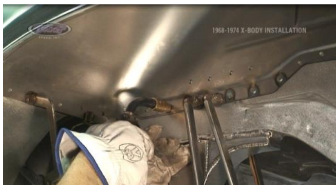
Figure 38 – Clamp and Weld to the Vehicle
