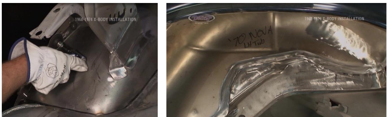
Figure 33 - Finish Grind Mini-Tub
