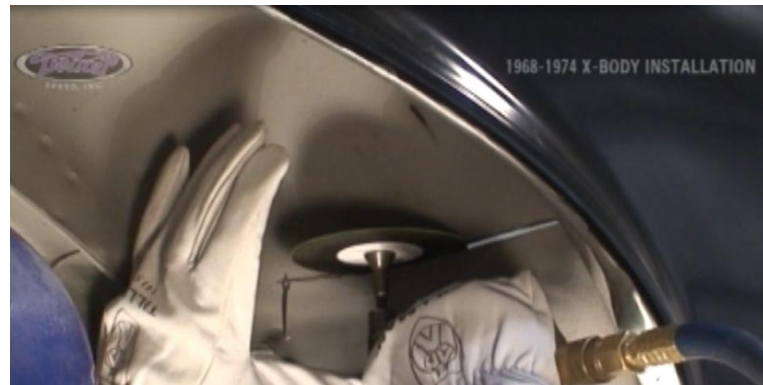
Figure 10 – Start Cutting the Stock Tub
