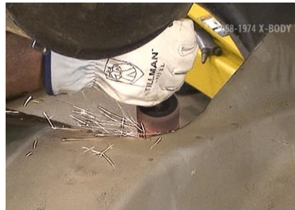
Figure 20 – Finish Cut and Grind Pre-Marked Lines
