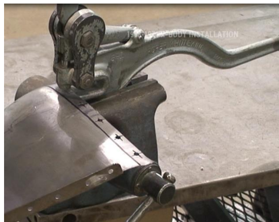
Figure 27 – Punch Spot Weld Holes
