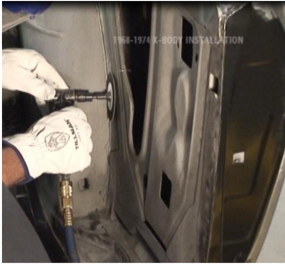
Figure 13 – Cut Pre-Marked Lines
