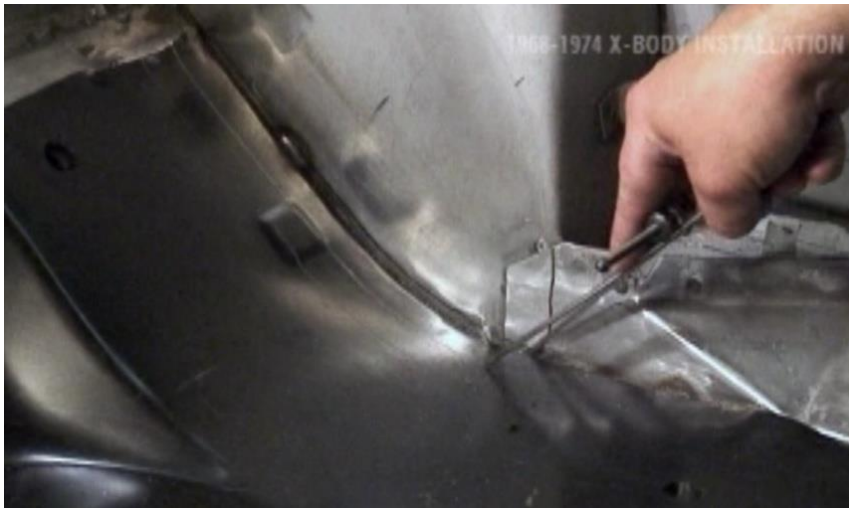
Figure 4 – Mark the Flange Bend Line
