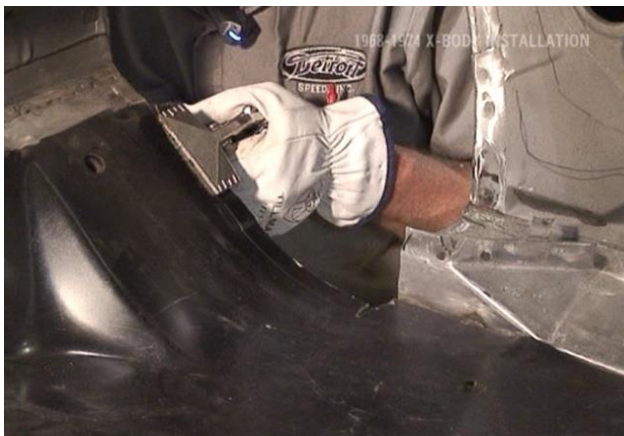
Figure 21 – Folding & Shaping of the Flange
