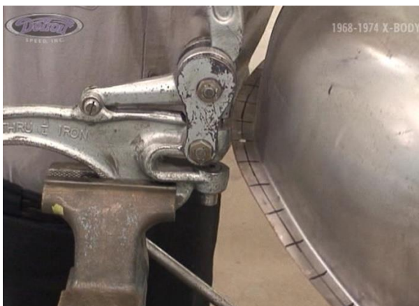
Figure 27 – Punch Spot Weld Holes
