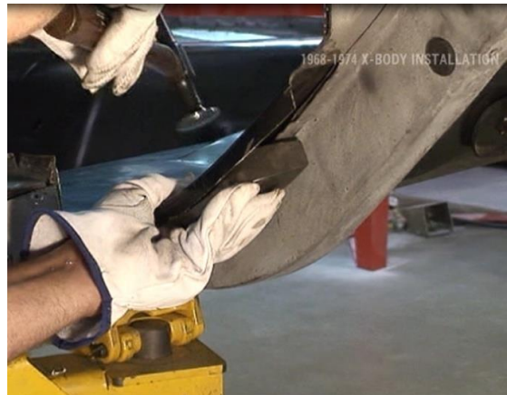
Figure 21 – Folding & Shaping of the Flange
