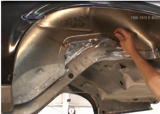
Figure 28 - Secure the Mini-Tub for Welding
