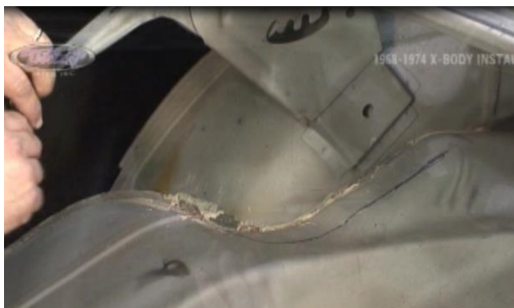
Figure 3 – Mark the Cut Lines
