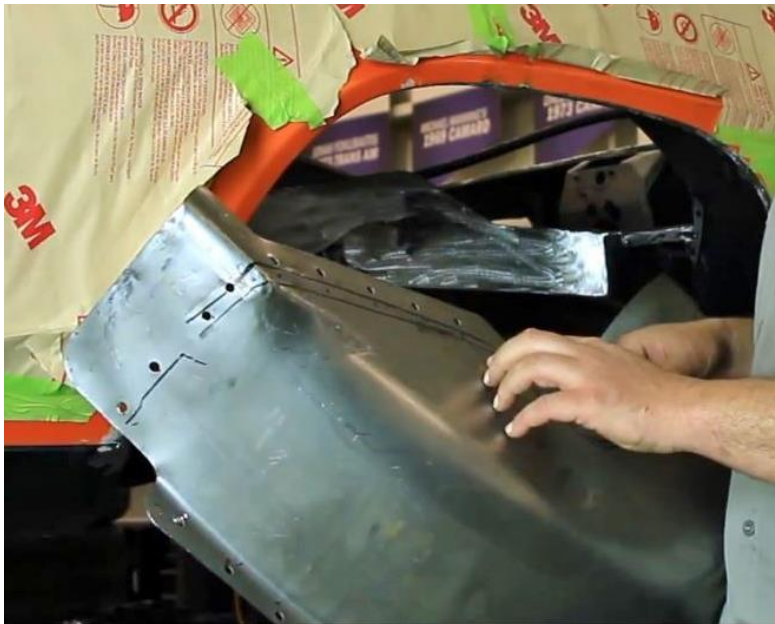
Figure 38 – Locate Plug Weld Holes
