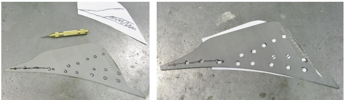
Figure 34 - Drill or Punch Plug Weld Holes
