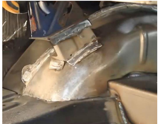
Figure 45 - Weld in Trunk Hinge Reinforcements.
