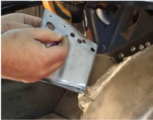
Figure 44 - Trim the Trunk Hinge Reinforcement
