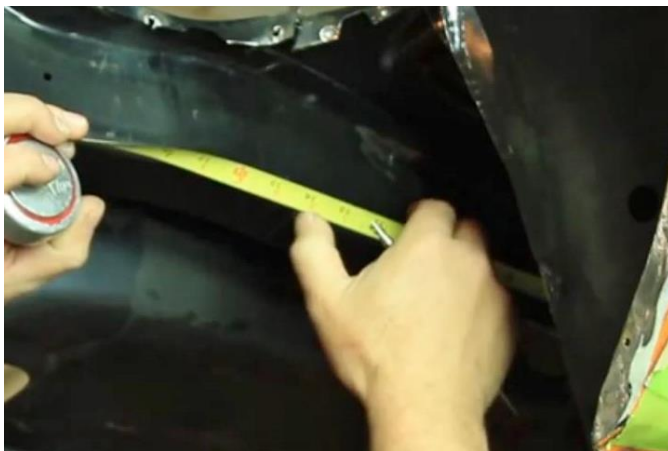
Figure 23 - Locate Bottom Frameraill Cut Template
