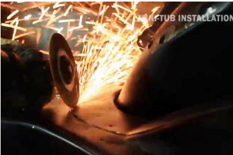
Figure 18 – Cutting the Trunk Floor
