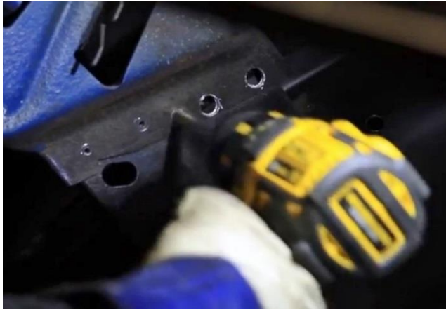
Figure 17 – Remove Decklid Reinforcement Bracket
