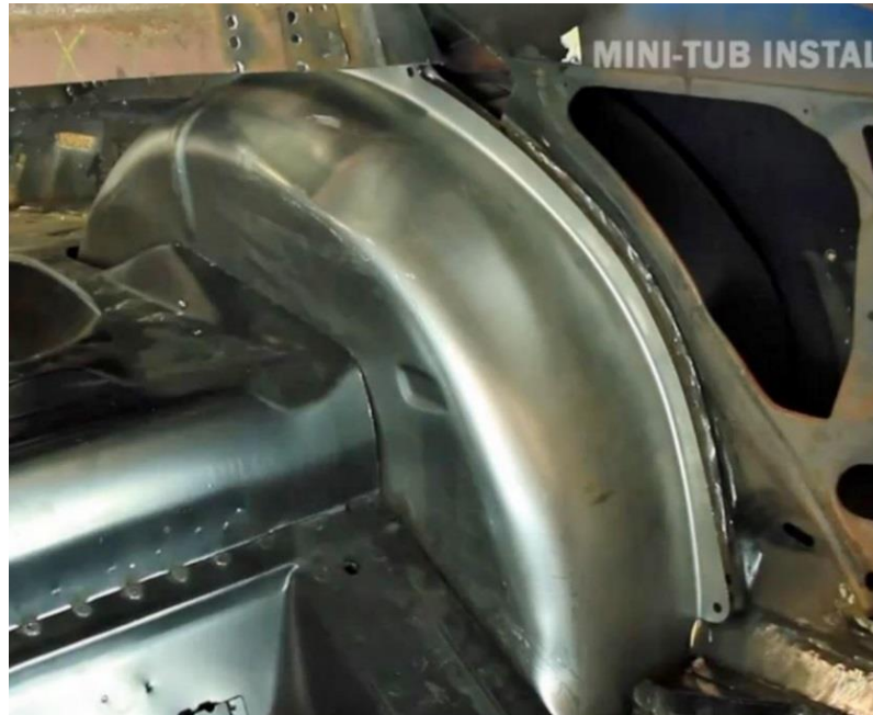
Figure 30 – Mock-up Detroit Speed Mini-Tub
