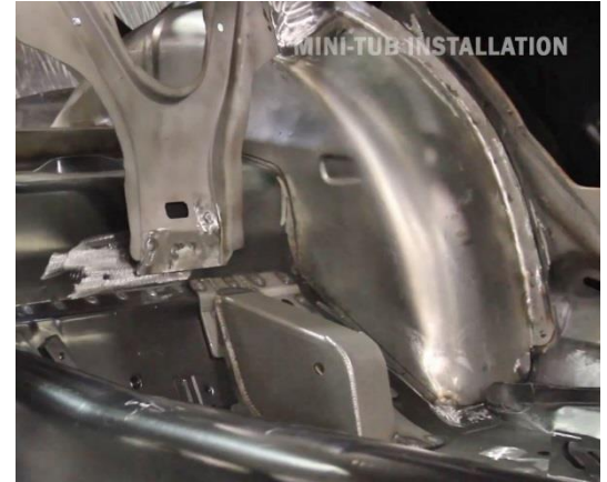
Figure 42 – Finished Detroit Speed Mini-Tub Installation
