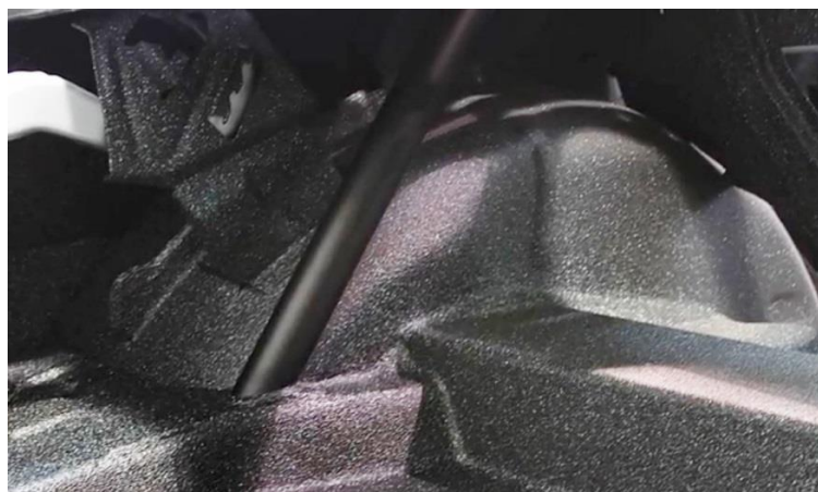
Figure 51 - Detroit Speed Mini-Tubs Completed
