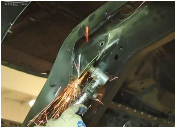
Figure 22 - Cutting the Frameraill Reinforcement
