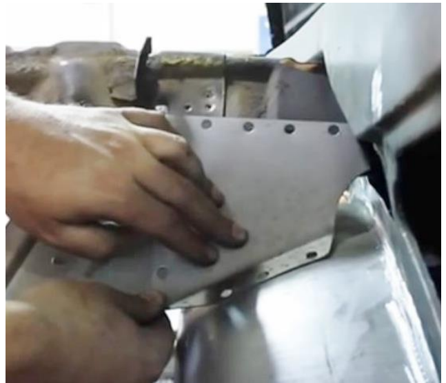
Figure 47 - Rear Seat Bracket Closeout
