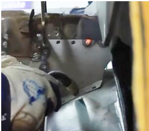
Figure 48 - Weld in Rear Seat Bracket Closeout
