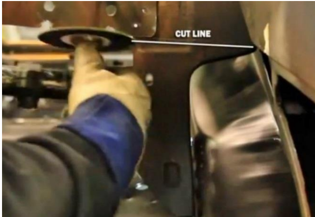
Figure 16 – Remove Section of Package Tray Reinforcement
