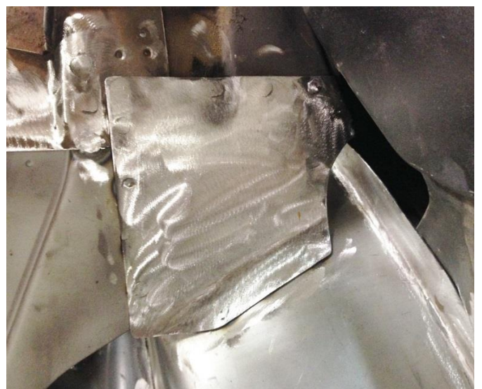
Figure 48 - Weld in Rear Seat Bracket Closeout
