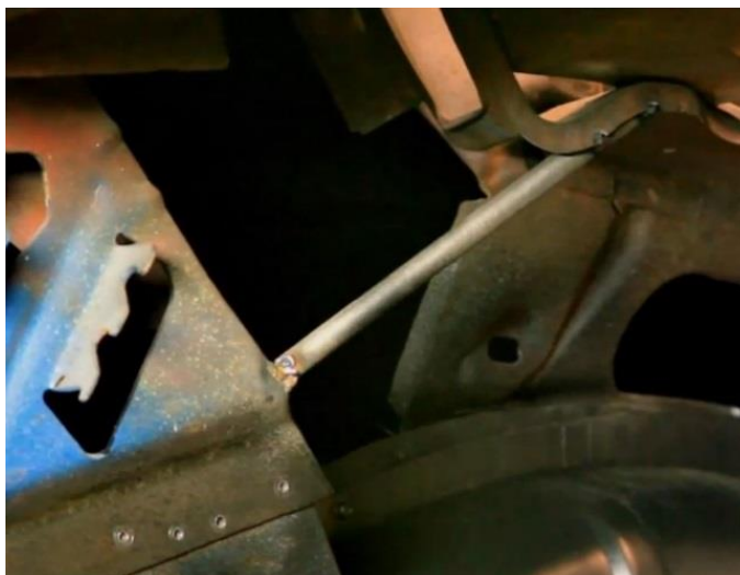
Figure 1 – Install Decklid Hinge Brace
