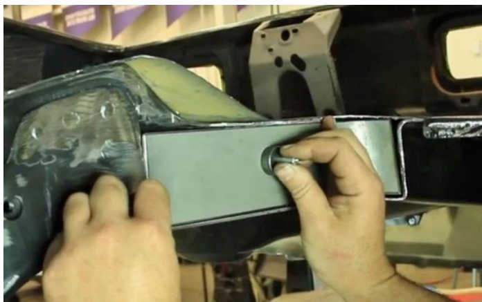
Figure 31 – Install Framerrail Closeout
