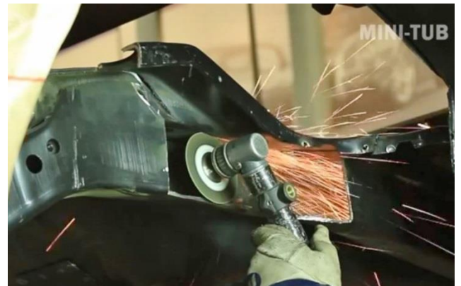
Figure 25 – Connect Cut Line to Framerrail
