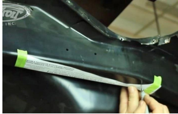
Figure 24 – Scribe Cut Line onto the Bottom Framerrail
