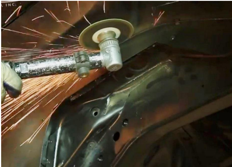
Figure 21 - Cutting the Inner Wheel Tub from the Trunk Floor
