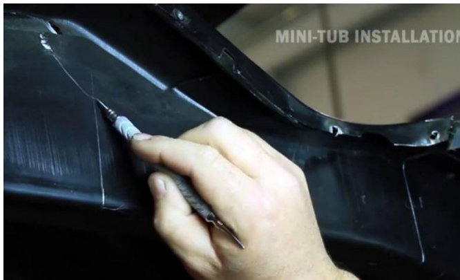
Figure 25 – Connect Cut Line to Framerrail
