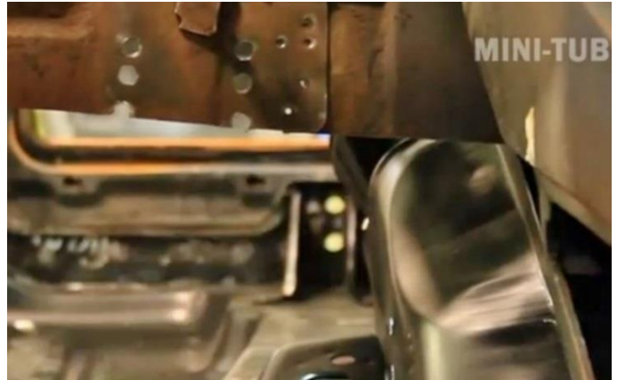
Figure 16 – Remove Section of Package Tray Reinforcement
