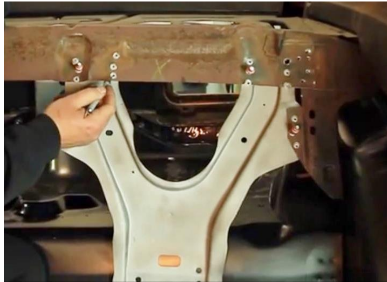
Figure 9 - Drill Out Spot Welds
