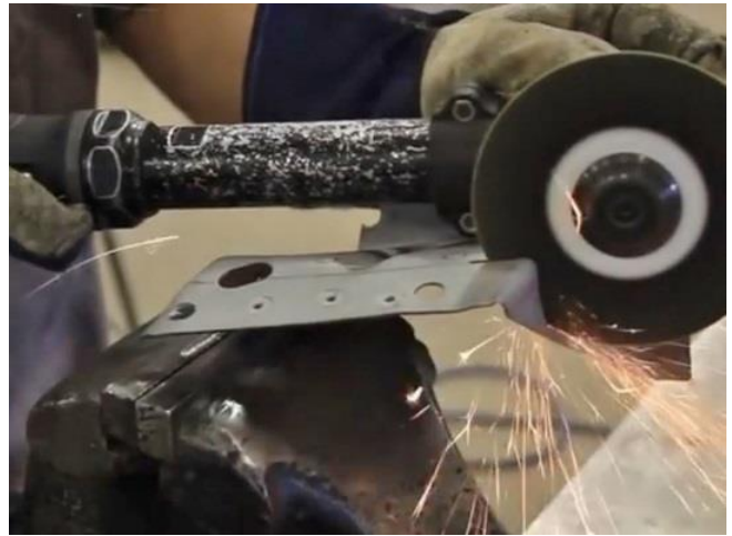
Figure 44 - Trim the Trunk Hinge Reinforcement
