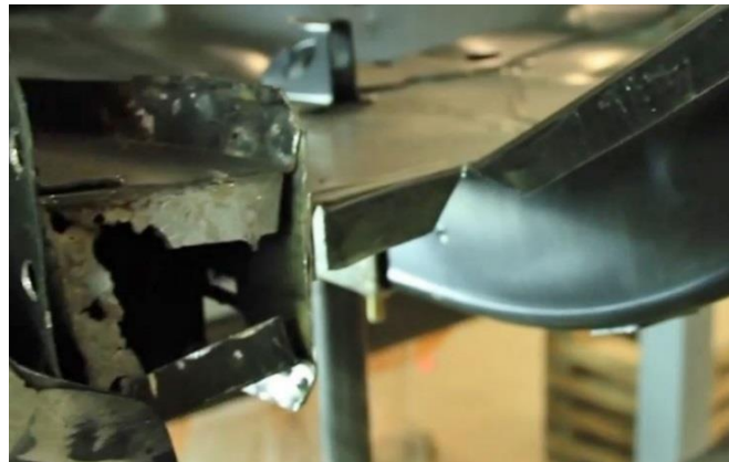
Figure 28 – Trim Rocker and Bend Fold Lines
