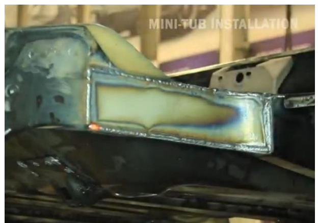
Figure 31 – Install Framerrail Closeout
