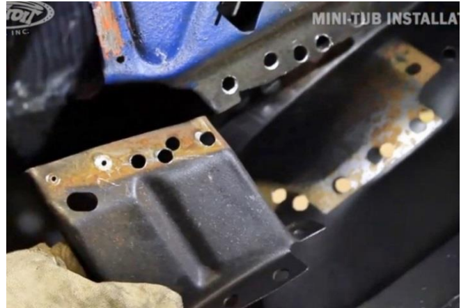
Figure 17 – Remove Decklid Reinforcement Bracket
