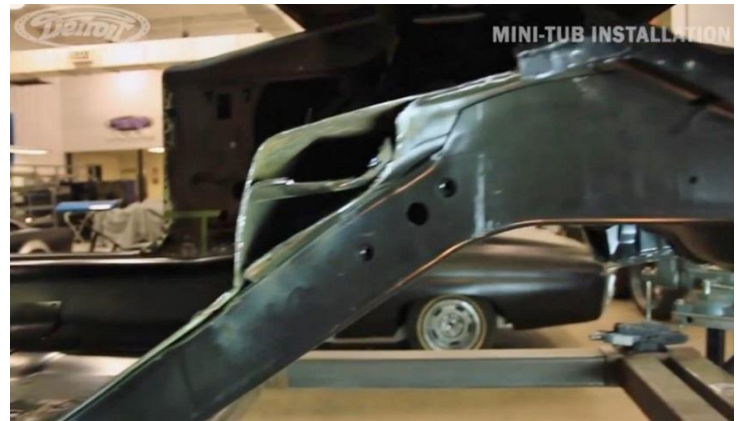
Figure 22 - Cutting the Frameraill Reinforcement
