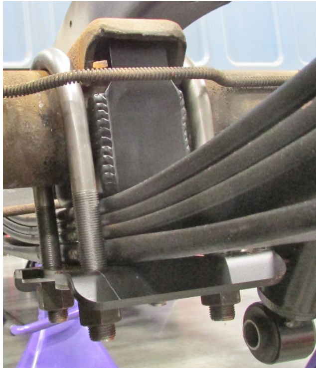
Figure 4 – Install Flip Kit Plate
