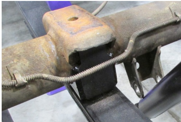
Figure 1 – Install Flip Kit Axle Pad
