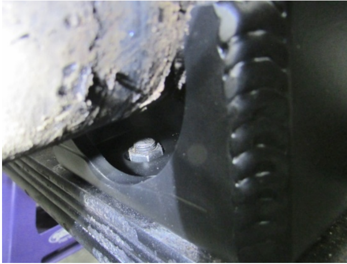
Figure 2 – Locate Axle Pad
