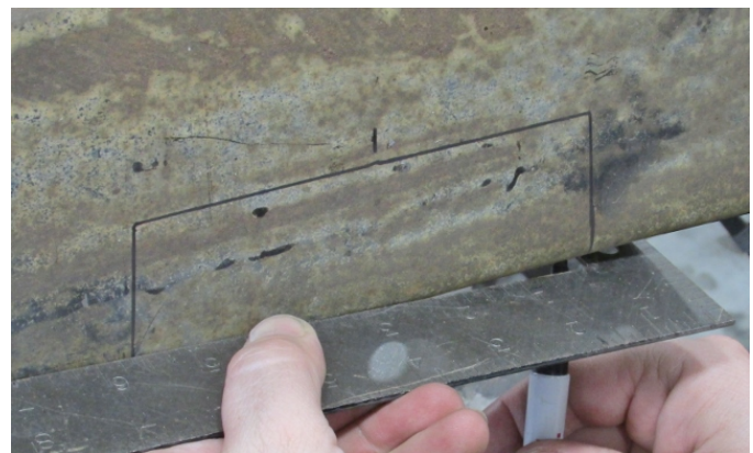
Figure 5 - Trace Frame Notch Cutout
