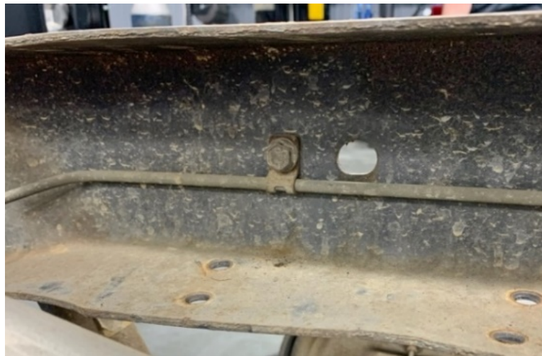
Figure 2 – Remove Brake Line Clamp
