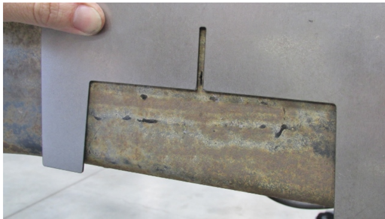
Figure 4 - Frame Notch Template
