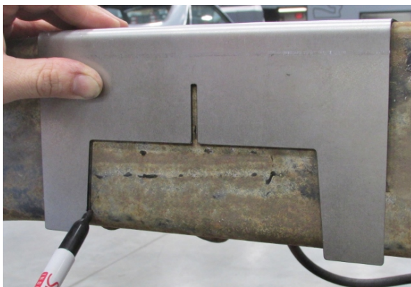
Figure 5 - Trace Frame Notch Cutout
