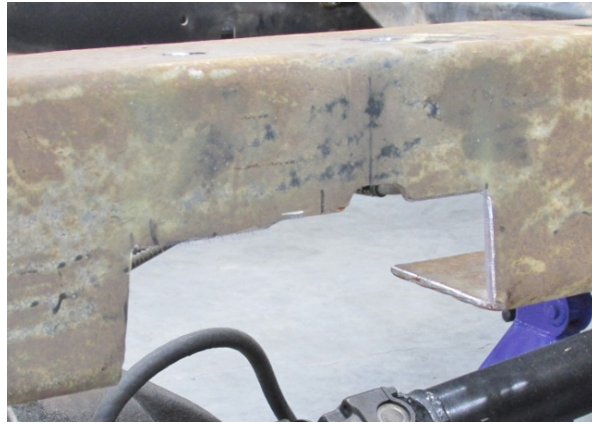
Figure 6 - Notch Frame Rail
