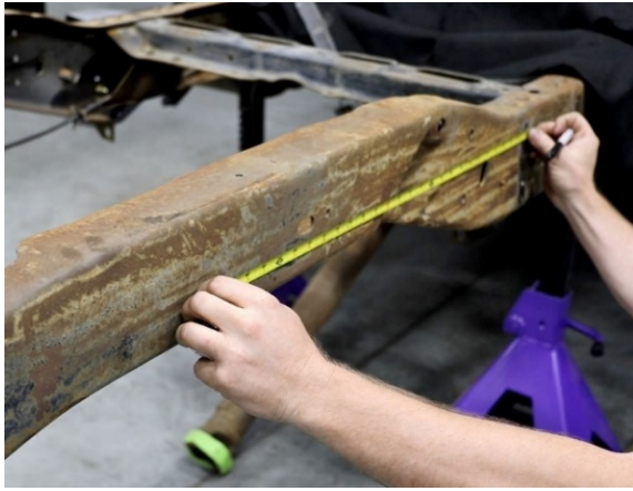
Figure 3 - Locate Notch Centerline
