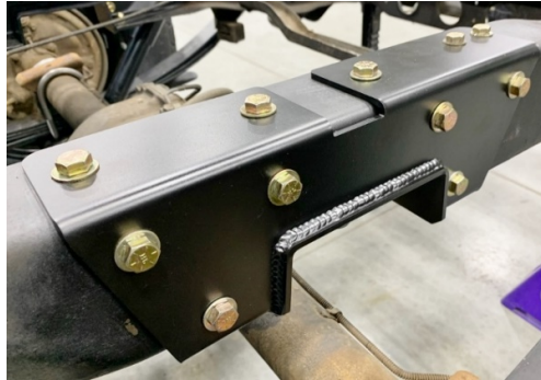
Figure 9 – Install Frame Notch Assemblies (RH, Passenger Side)
