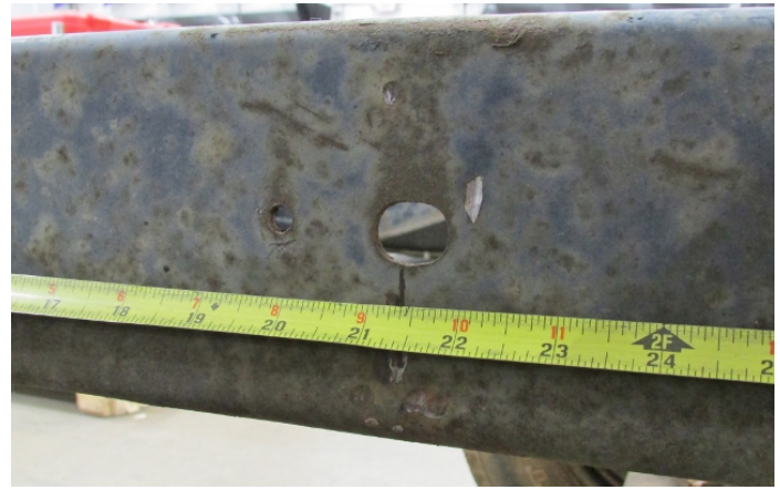
Figure 3 - Locate Notch Centerline
