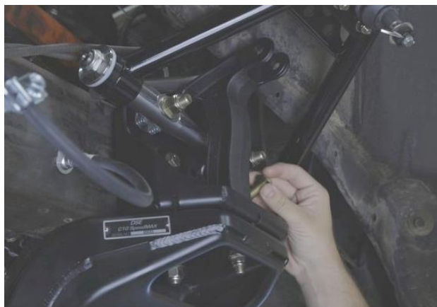
Figure 50 - Install Upper Coilover Mount
