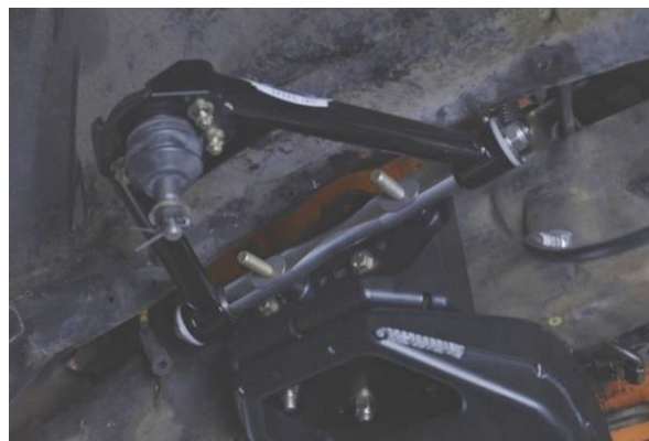
Figure 45 - Install Upper Control Arms
