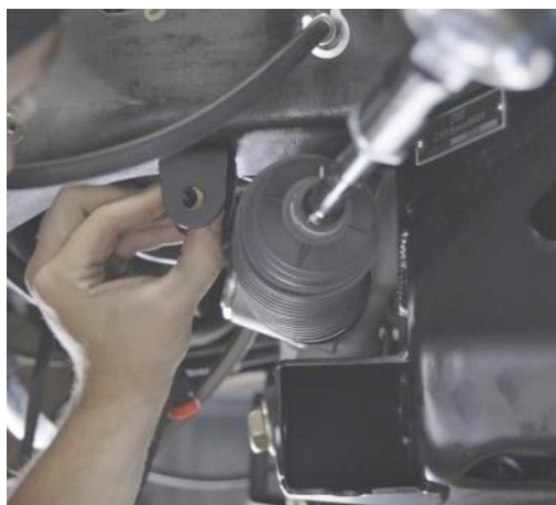
Figure 64 – Install Sway Bar Mount Crush Sleeve
