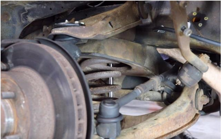
Figure 14 - Remove Cradle Hardware
