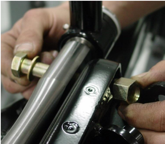
Figure 4c - Installing the Hardware
