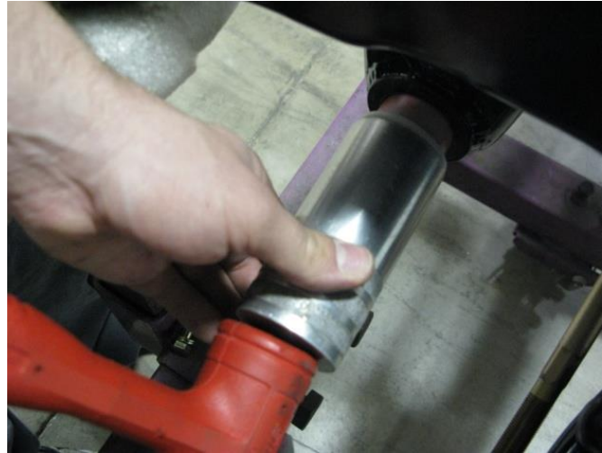
Figure 18 - Fully Installing the Bushings
