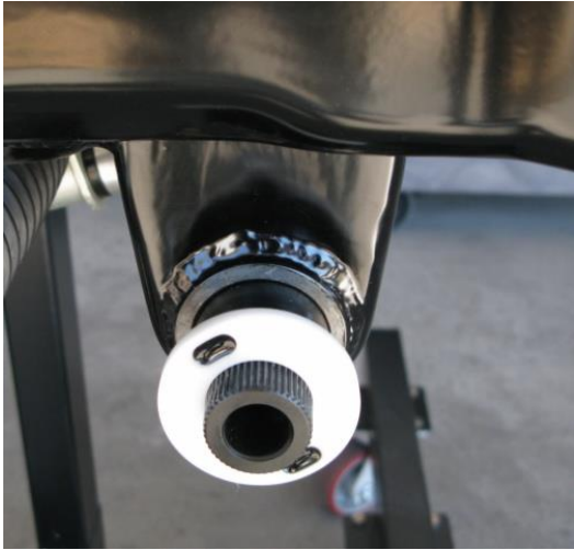
Figure 17 - Installing Bushing & Sway Bar
