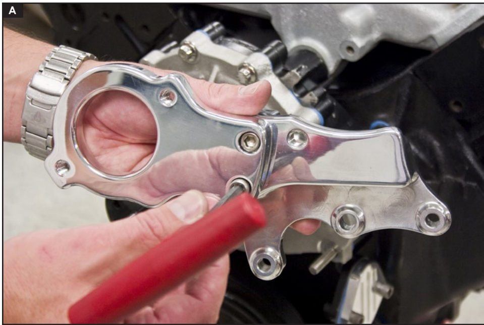
Figure 3: Install Power Steering Bracket
