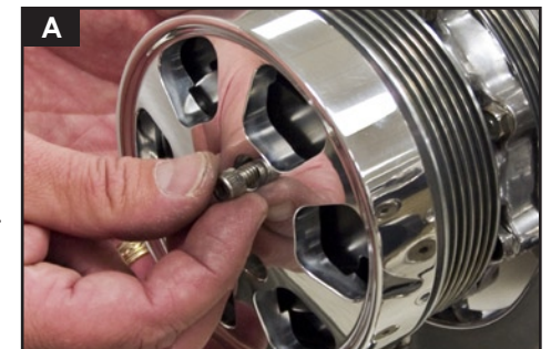
Figure 9: Install AC Compressor Cover
