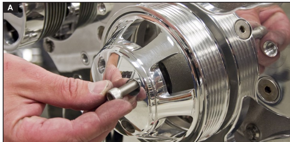
Figure 13: Install Water Pump Pulley
