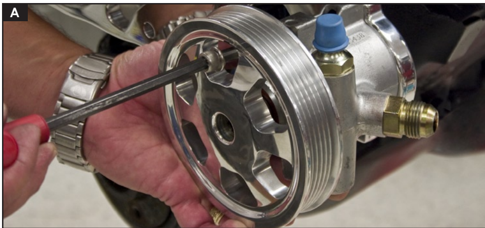
Figure 11: Install Power Steering Pump & Pulley
