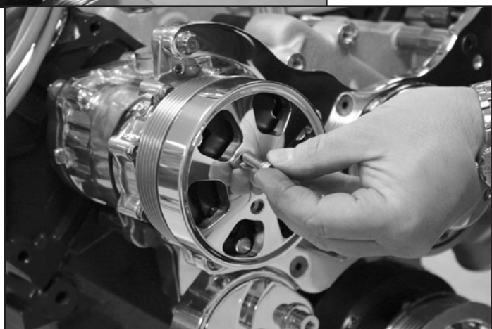
Figure 11: Install Water Pump Pulley & A/C Compressor Clutch Cover
