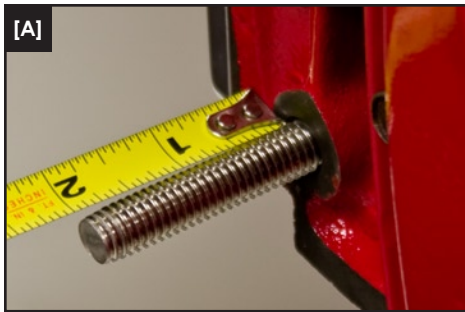
Figure 1: Install Block Mounting Studs
