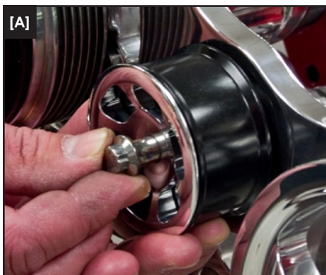
Figure 11: Install Idler Pulleys
