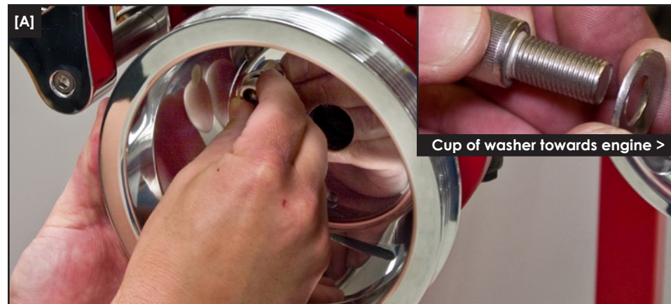
Figure 10: Install Crankshaft Pulley
