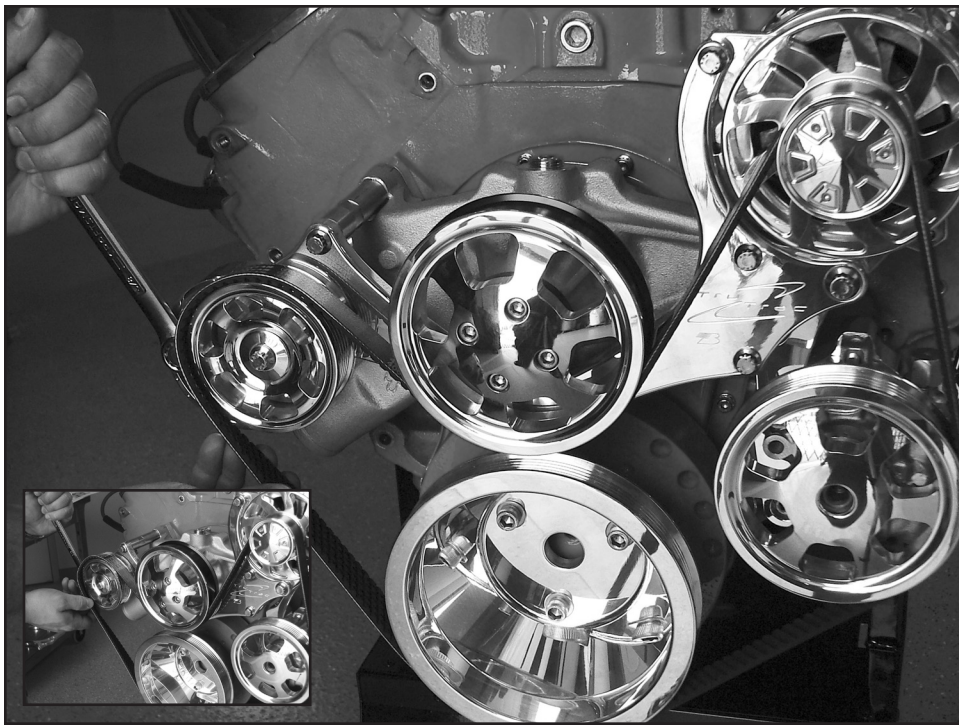
Figure 15: Install Serpentine Belt
