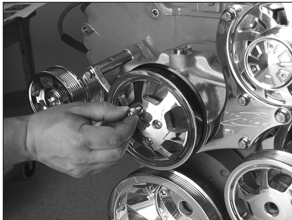
Figure 14: Install Water Pump Pulley onto Pump
