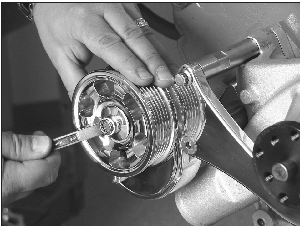
Figure 13: Install Tensioner Pulley
